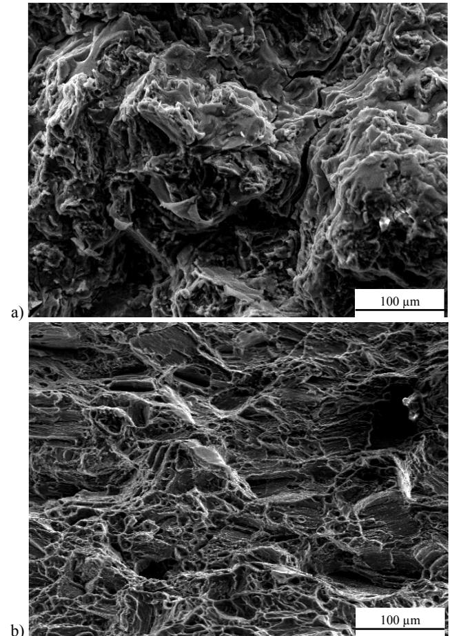
Fig.4. The fracture surface of tensile test alloy MCMgAl9Zn1: a) without heat treatment – as-cast, b) after aging treatment
