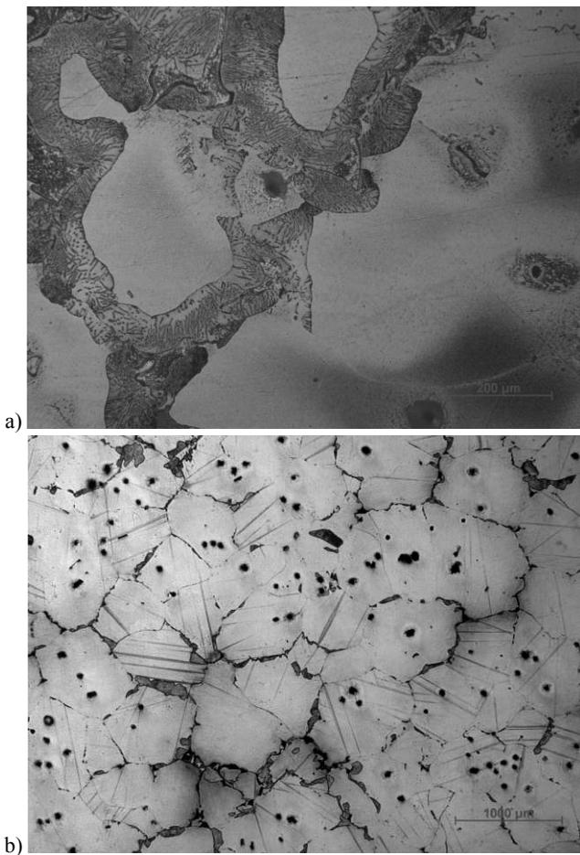
Fig 3. Microstructure alloy MCMgAl9Zn1: a) without heat treatment – as-cast, b) after aging treatment
