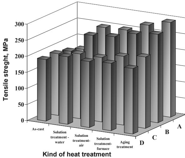
Fig. 2. The results of Tensile strength magnesium casting alloys: A) MCMgAl12Zn1, B) MCMgAl9Zn1, C) MCMgAl6Zn1, D) MCMgAl3Zn1
