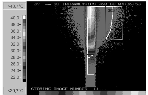
Fig. 6. Thermographic image of sample after 1 190 000 fatigue cycles of fatigue testing 20 seconds after heating
