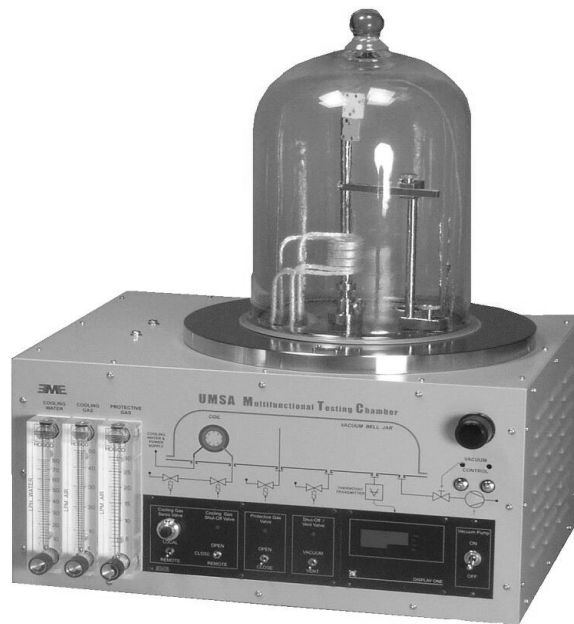
Fig. 1. Multifunctional, Environmental UMSA Platform Testing Chamber (the University of Windsor, Canada). This chamber is the main functional UMSA component
