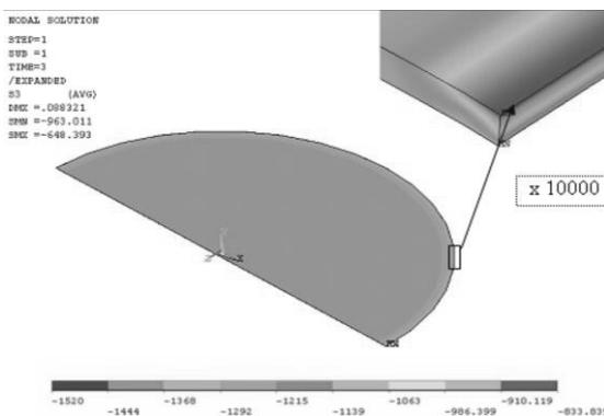
Fig. 1. Distribution of the simulated compression stresses in the Ti+Ti(C<sub>x</sub>N<sub>1-x</sub>) coatings in working atmosphere including 75% N<sub>2</sub> i 25% CH<sub>4</sub>. (coating thickness g=6,4 μm, process temperature 460°C)
