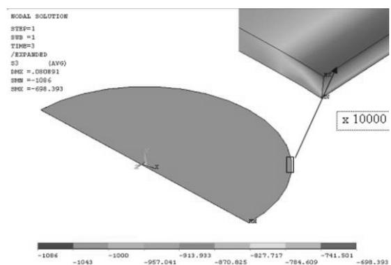
Fig. 2. Distribution of the simulated compression stresses in the Ti+Ti(C<sub>x</sub>N<sub>1-x</sub>) coatings in working atmosphere including 25% N<sub>2</sub> i % 75CH<sub>4</sub>. (coating thickness g=4,7 μm, process temperature 500°C)
