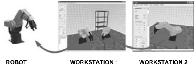
Fig. 7. The ROBO application operating in mixed mode. Workstation 1 controls the real and the virtual robot
