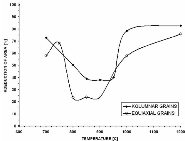
Fig. 1. The hot ductility curves
