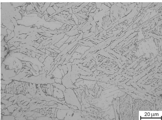
Fig. 5. Microstructure of a sample deformed at 900°C
