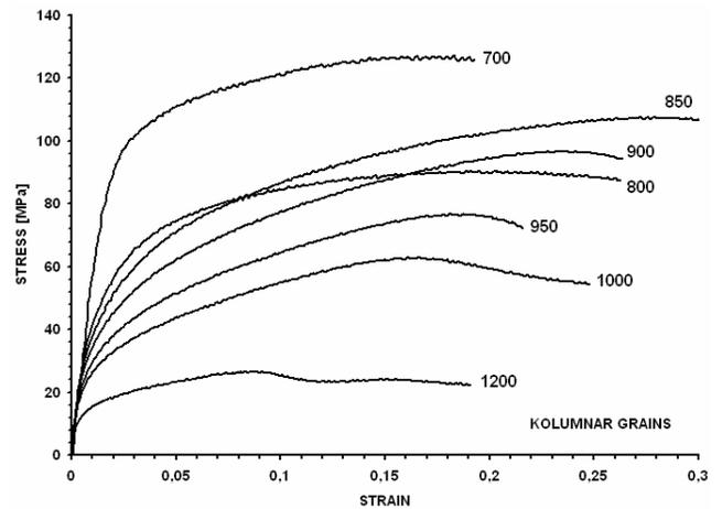
Fig. 2. True flow curves for columnar grained samples deformed with 0.01/s strain rate
