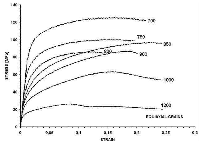
Fig. 3. True flow curves for equiaxial grained samples deformed with 0.01/s strain rate
