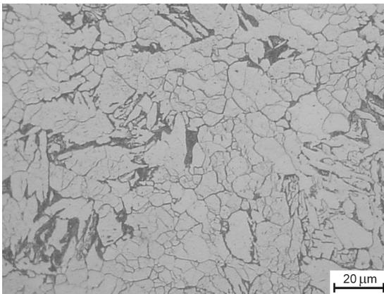
Fig. 4. Microstructure of a sample deformed at 800°C
