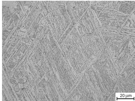
Fig. 6. Microstructure of a sample deformed at 1200°C
