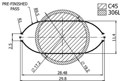
Fig. 1. Shape and dimensions of the pre-finished pass and dimension of initial band
