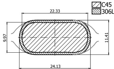
Fig. 3. Shape and dimensions of the bimetallic flat oval band obtained in numerical modelling – cross-section
