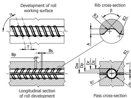
Fig. 2. Shape and dimensions of the round ribbed finished pass
