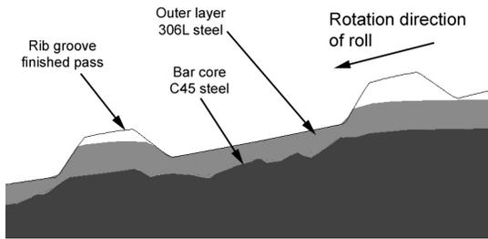
Fig.6. Forming of bimetallic bar ribs in ribbed finished pass
