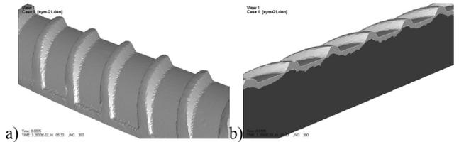
Fig. 4. Bimetallic round ribbed bar model 16 mm: a) view of bar outer layer, b) view of bar longitudinal section
