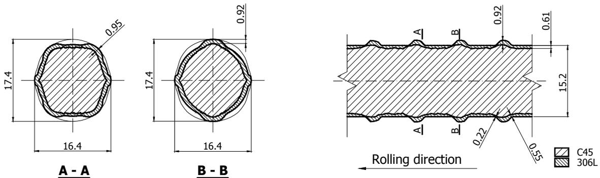
Fig. 5. Shape and dimensions bimetallic round ribbed bar 16 mm obtained in computer simulation
