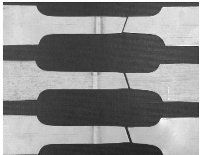
Fig. 2. A view of butt joints of austenitic steel AISI 321 sheets 1,0 [mm] thick welded by the high power diode laser HPDL ROFIN DL 020 after static tensile test. Broken in base material
