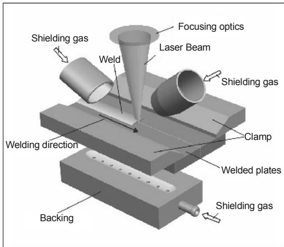
Fig. 1. A view of the device for mounting of welded joints with a copper backing plate
