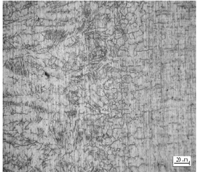
Fig. 5. Microstructure of butt joints of austenitic steel AISI 321 sheets 0,5 [mm] thick welded by the high power diode laser HPDL ROFIN DL 020 at laser power 0,6 [kW] and welding speed 0,6 [m/min]; (from left) weld metal, very narrow heat affected zone and austenitic structure of the base material, etched by iron chloride  $\text{FeCl}_3$ , magnification 200x
