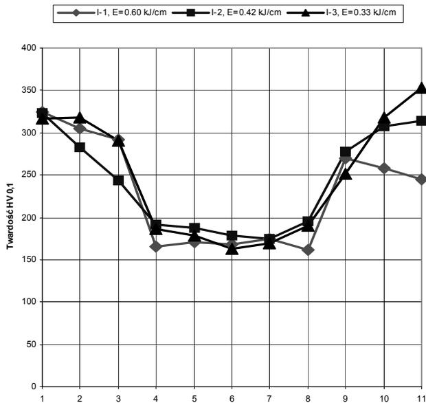
Fig. 4. Microhardness distribution on the cross-section of the butt joints of austenitic steel AISI 321 sheets 1,0 [mm] thick welded by the high power diode laser HPDL
