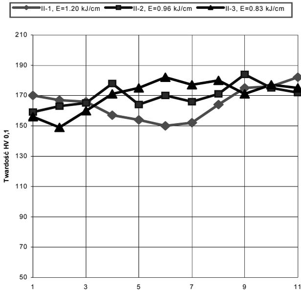
Fig. 3. Microhardness distribution on the cross-section of the butt joints of austenitic steel AISI 321 sheets 0,5 [mm] thick welded by the high power diode laser HPDL
