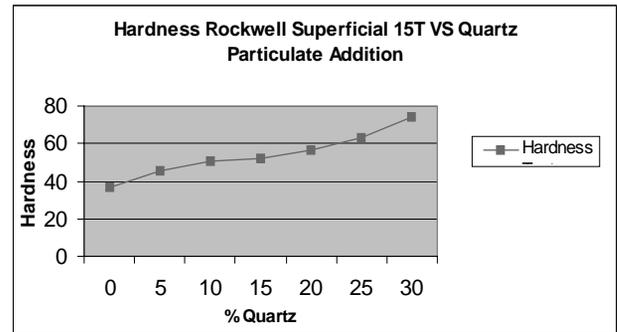
Fig. 6. Hardness value of the processed composites increases with the increase in addition of quartz particulate by volume fraction %
