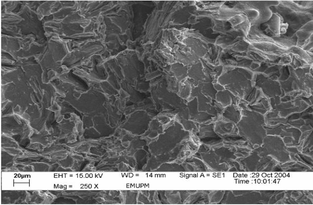
Fig. 7. Fractograph of 5% SiO<sub>2</sub> particulate reinforced in SiO<sub>2</sub>-LM6 alloy matrix composite at 250X magnification by SEM after tensile testing
