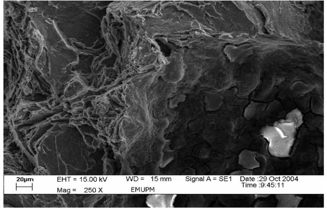
Fig. 11. Fractograph of 25% SiO<sub>2</sub> particulate reinforced in SiO<sub>2</sub>-LM6 alloy matrix composite at 100X magnification by SEM after tensile testing which shows the peeled out particulate
