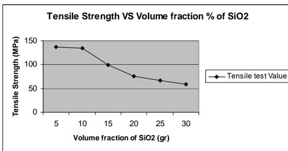
Fig. 4. Average tensile strength versus volume fraction of SiO<sub>2</sub>
