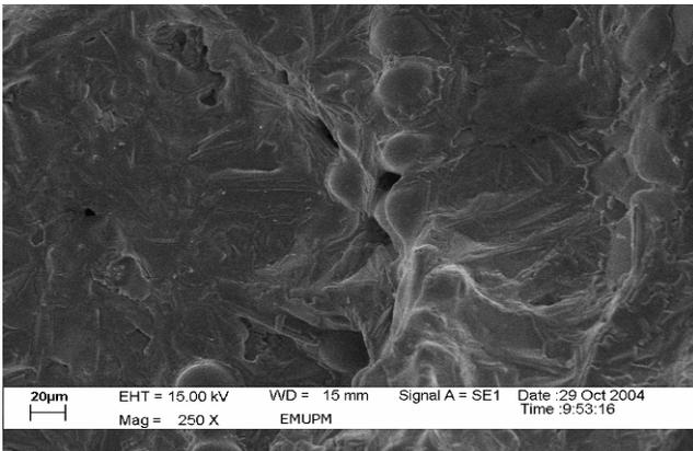
Fig. 9. Fractograph of 15% SiO<sub>2</sub> particulate reinforced in SiO<sub>2</sub>-LM6 alloy matrix composite at 250X magnification by SEM after tensile testing which shows intergranular movement
