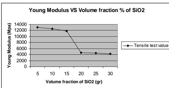
Fig. 5. Average young modulus versus volume fraction of SiO<sub>2</sub>
