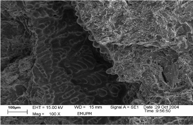
Fig. 8. Fractograph of 10% SiO<sub>2</sub> particulate reinforced in SiO<sub>2</sub>-LM6 alloy matrix composite at 100X magnification by SEM after tensile testing
