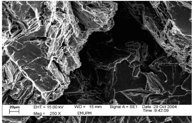
Fig. 12. Fractograph of 30% SiO<sub>2</sub> particulate reinforced in SiO<sub>2</sub>-LM6 alloy matrix composite at 250X magnification by SEM after tensile testing
