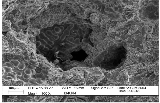
Fig. 10. Fractograph of 20% SiO<sub>2</sub> particulate reinforced in SiO<sub>2</sub>-LM6 alloy matrix composite at 100X magnification by SEM after tensile testing which shows the crack propagation in the ductile matrix
