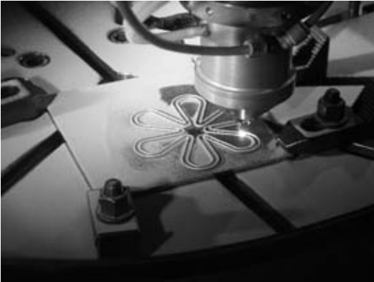
Fig. 2. Manufacturing of special shaped product by fiber laser using LENS Technology principle
