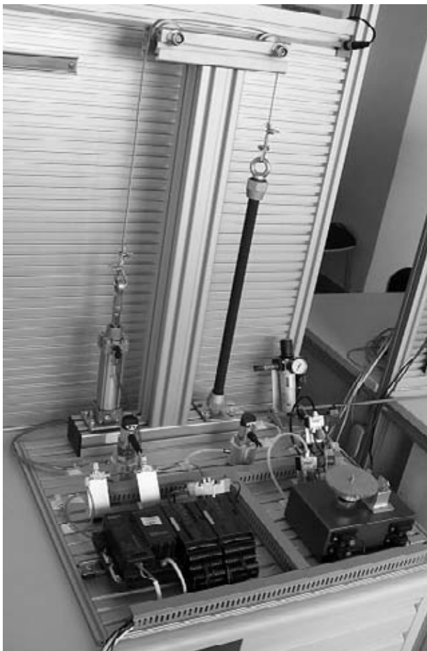
Fig. 2. The view of the stand for Fluidic Muscle investigations
