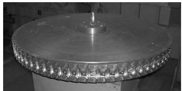
Fig. 8. Milling head with sintered carbides
