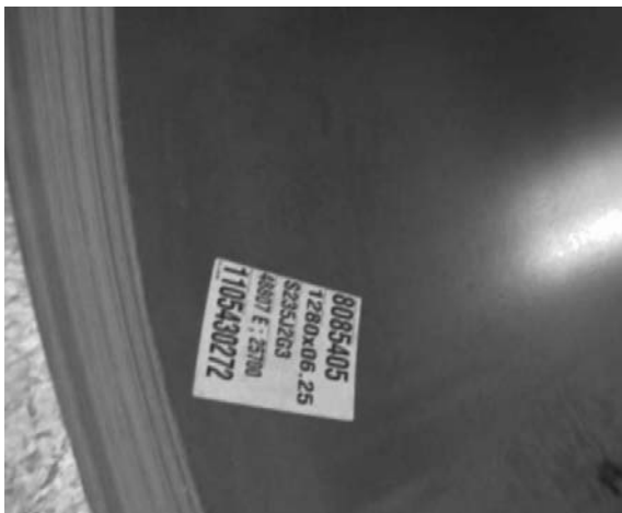
Fig. 2. Specification of a metal coil
