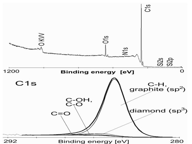
Fig. 7. An overall XPS spectrum from the surface of the amorphous a-C coating deposited by means of a discontinuous CAE process onto the surface of a pure Si substrate (on the top) and the carbon C1s peak from that figure resolved into different components including the diamond-like  $sp^3$  and the graphite-like  $sp^2$  ones (lower down)
