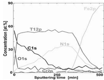
Fig. 6. In depth concentration profiles of a thin ( $\sim 150nm$ ) gradient  $Ti_xN_y$  coating on tempered T1 HSS steel with a continuous change of concentration of carbon atoms from 0 at.% at the substrate to  $\sim 50$  at.% at the top of the coating and an opposite change of concentration of nitrogen atoms: from about 36 at.% to 0 at.%
