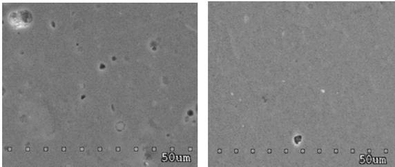
Fig. 2. SEI morphology of the surface of two gradient  $Ti_xN_y$  coatings deposited by means of a continuous CAE process onto the diffusion hardened Ti6Al4V alloy without (photo on the left) and with magnetic filtering of microdroplets (that on the right)
