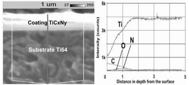
Fig. 5. SEI image (left) of a fracture of the gradient  $Ti_xN_y$  coating on diffusion hardened (with oxygen atoms) Ti6Al4V substrate. The arrow is marking an area and direction of the EDS line scan pro-files of concentration of the elements Ti, C, O and N, which are shown on the right hand side
