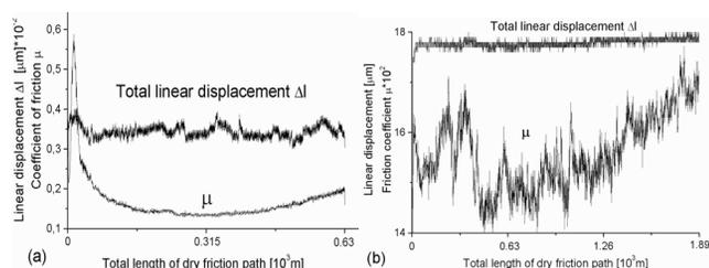
Fig. 8. Dry friction coefficient and wear against a ball from bearing steel of diffusion hardened Ti6Al4V alloy with a gradient  $Ti_xN_y$  layer and the amorphous a-C coating as the top layer (on the left) and the same substrate with a gradient a-C:H(Ti)<sup>†</sup> coating as the top layer (on the right)
