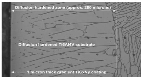
Fig. 3. SEI image of the microstructure of the two-phase  $\alpha+\beta$  Ti6Al4V substrate after diffusion hardening and coating with  $\sim 1\mu m$  gradient  $Ti_xN_y$  layer with use of CAE process
