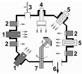
Fig. 1. Scheme of the equipment of the working chamber of a multi-purpose installation for deposition of different PVD coating systems: 1- two independent 4 kW arc guns for continuous CAE process; 2- four independent 4kV Ar ion guns; 3- gas flow control system; 4- 10kW mag neutron gun; 5- two independent arc sources for discontinuous CAE pro-cess; 6- connection to vacuum pumps; 7- rotary table for specimens with digital position control system
