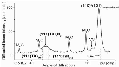
Fig. 4. XRD diffraction profile from the surface of  $1\mu m$  thick gradient  $Ti_xN_y$  coating deposited onto tempered T1 HSS substrate
