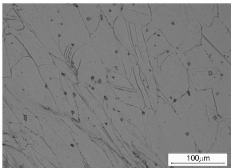
Fig. 6. Optical micrograph for the sample of In718 deformed at 900°C, strain rate of  $10^{-4} \text{ s}^{-1}$
