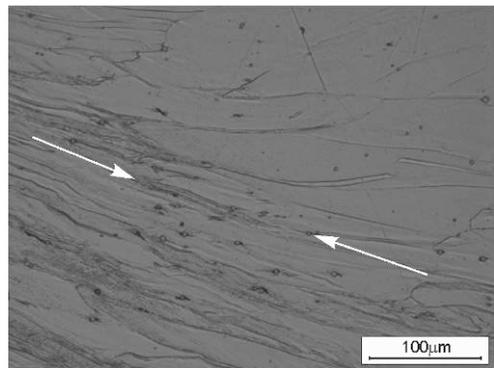
Fig. 4. Microstructure of the sample deformed at 720°C, strain rate of  $4 \cdot 10^{-4} \text{s}^{-1}$
