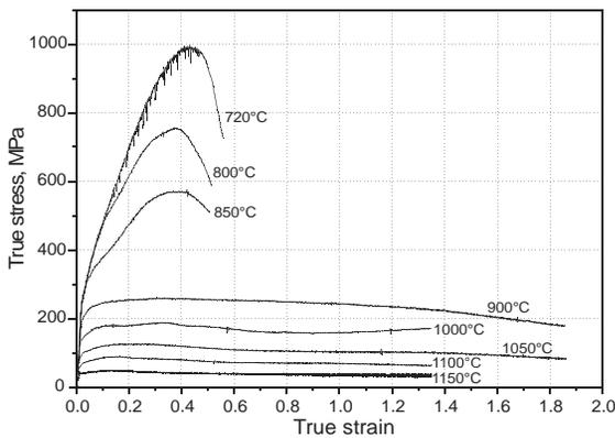
Fig. 1. True stress-true strain curves for Inconel 718 alloy deformed at different temperatures and a strain rate of  $10^{-4} \text{s}^{-1}$  (the deformation temperature was indicated in the figure)
