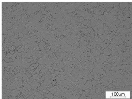
Fig. 7. Optical micrograph for the sample of In718 deformed at 1050°C, strain rate of  $4 \cdot 10^{-4} \text{ s}^{-1}$
