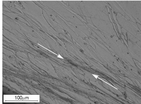
Fig. 3. Microstructure of the sample deformed at 720°C, strain rate of  $10^{-4} \text{s}^{-1}$
