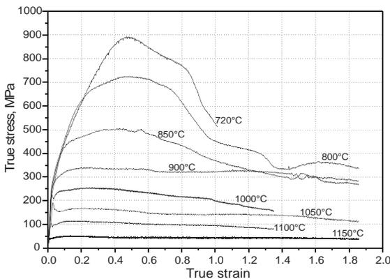
Fig. 2. True stress-true strain curves for Inconel 718 alloy deformed at different temperatures and a strain rate of  $4 \cdot 10^{-4} \text{s}^{-1}$  (the deformation temperature was indicated in the figure)
