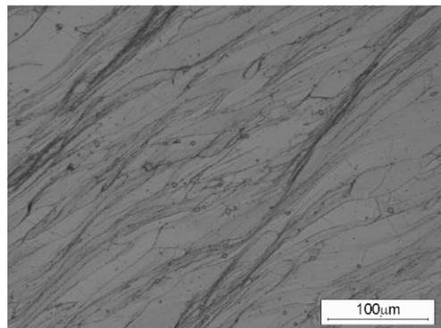
Fig. 5. Optical micrograph for the sample of In718 deformed at 850°C, strain rate of  $4 \cdot 10^{-4} \text{s}^{-1}$
