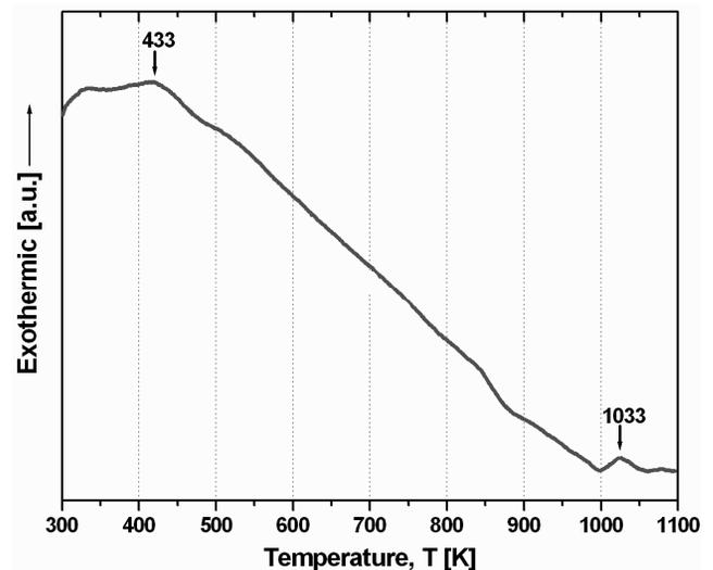
Fig. 2. DTA pattern of  $\text{Fe}_2\text{O}_3$  and  $\text{BaCO}_3$  mixture after 50 hours of milling process
