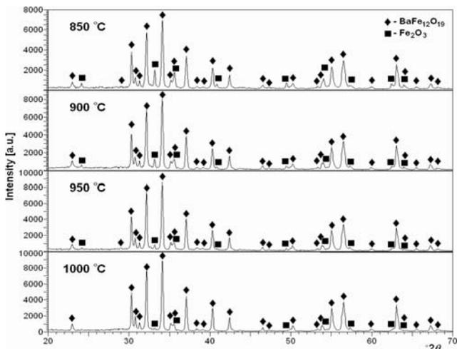
Fig. 4. X-ray diffraction patterns of  $\text{Fe}_2\text{O}_3$  and  $\text{BaCO}_3$  mixture after 50 hours of milling and annealing at 850, 900, 950 and 1000°C
