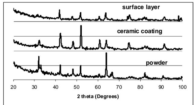
Fig. 4. Diffraction patterns obtained for ceramic powder, plasma sprayed coating and for alloyed surface layer
