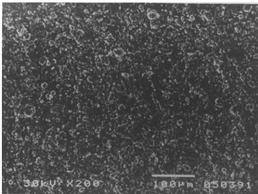
Fig. 1. Microstructure of plasma sprayed ceramic coating, magnification 200x
