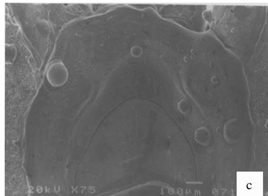
Fig. 2. Microstructure in remelting paths which occurred for the following rates of irradiation: a)  $V_1=750$  mm/min, b)  $V_2=800$  mm/min, c)  $V_3=850$  mm/min
