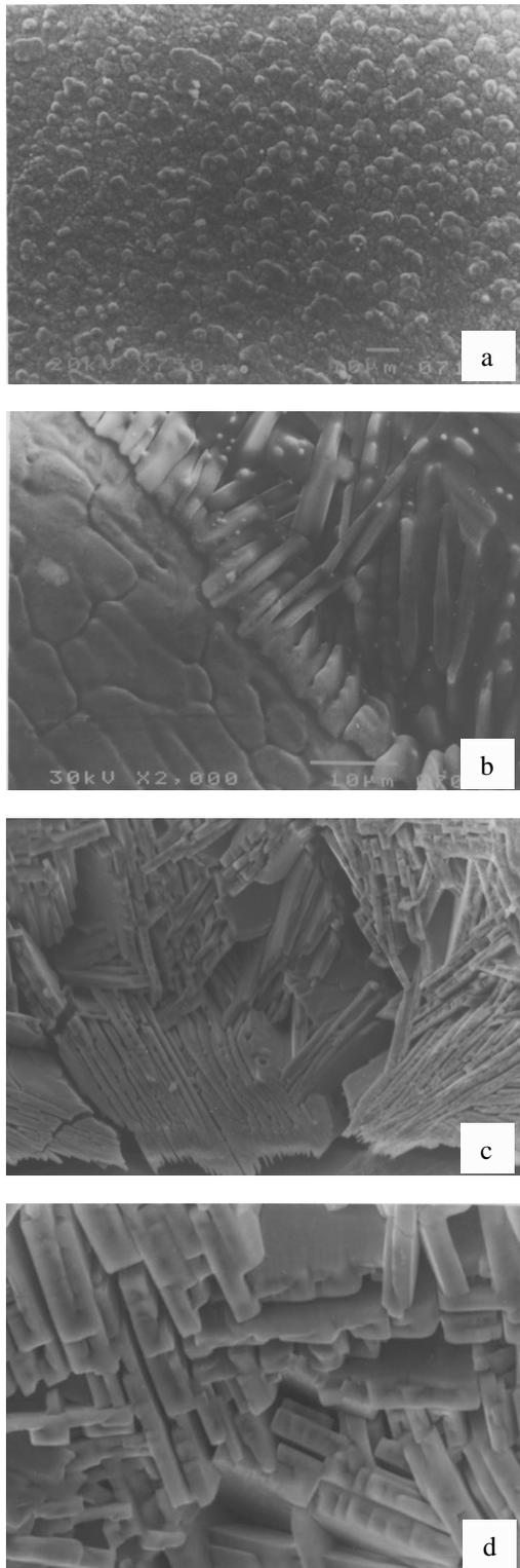
Fig. 3. Microstructure of the zones created as a result of the applied laser treatment, a) remelted path, b) borderline of the remelted zone and outflow zone, c,d) outflow
