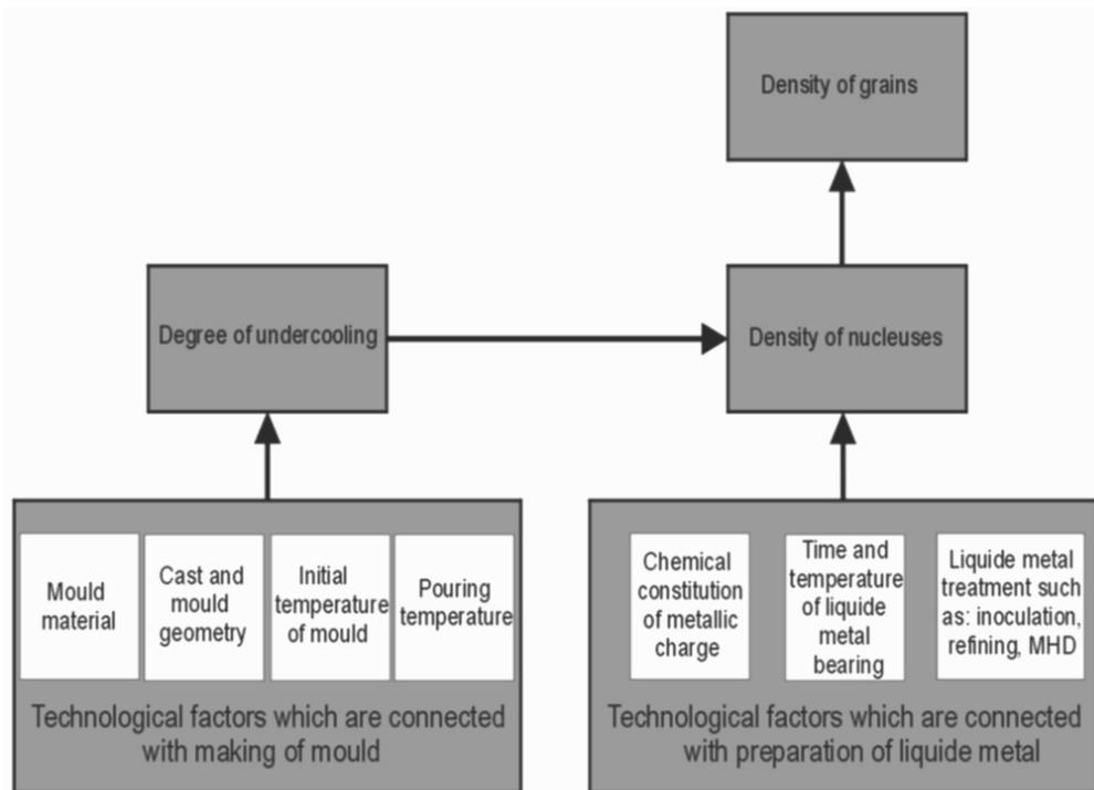
Fig. 1. Influence of technological parameters on structure of casting [1]
