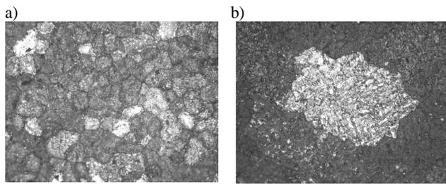
Fig. 4. Microstructure of aluminium EN AW-Al99.5 – 100x: a – area 1 from Fig. 3b, b – area 2 from Fig. 3b
