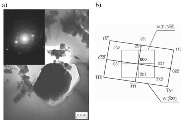
Fig. 5. a) Diffraction and structure of thin foil from EN AW-Al99.5 after inoculation with (Ti+B) – 30000x, b) solution of the diffraction pattern from Fig. 5a
