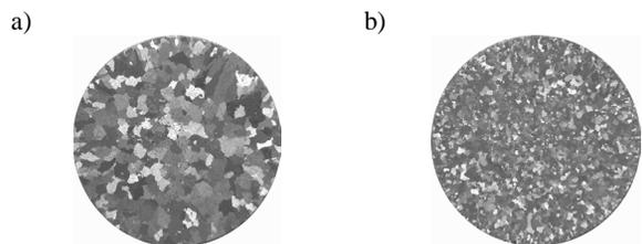
Fig. 2. Macrostructure of aluminium EN AW-Al99.5: a – sample 3, b – sample 4
