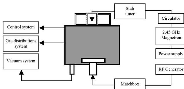
Fig. 1. Schematic of deposition system used in presented work
