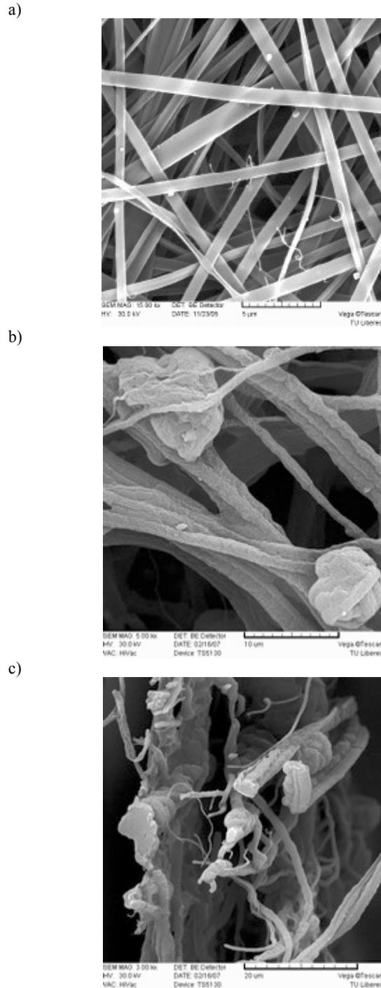
Fig. 3. SEM image of nanofiber textile a) uncovered, b) covered by carbon coatings, c) cross section of nanofibers covered by carbon coatings
