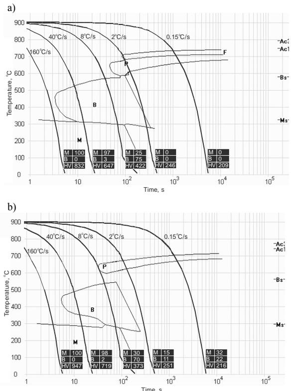
Fig. 2. Comparison of the CCT diagram with marked structural participation of martensite (M) and bainite (B) and hardness of steel (HV) for five different cooling rates: a) accepted as a model (C45E), b) suggested by the neural network (C60E)
