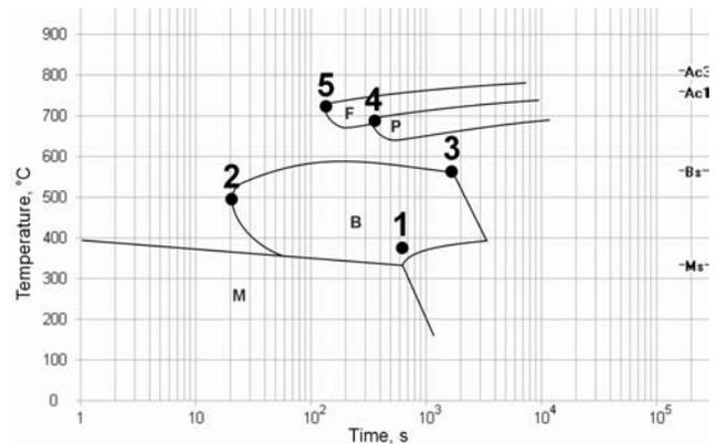
Fig. 1. CCT diagram with characteristic points marked
