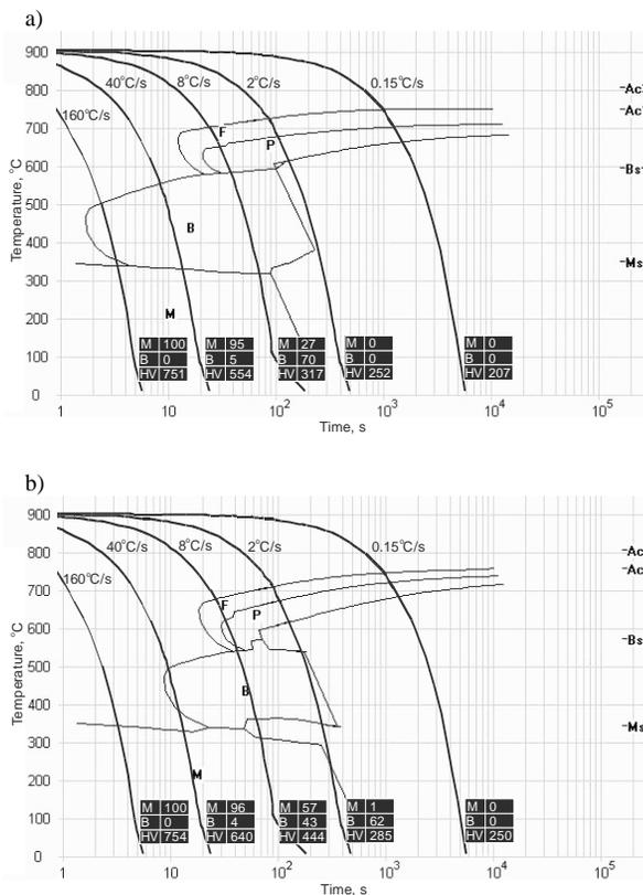
Fig. 3. Comparison of the CCT diagram with marked structural participation of martensite (M) and bainite (B) and hardness of steel (HV) for five different cooling rates: a) accepted as a model (C45E), b) suggested by the neural network (41Cr4)
