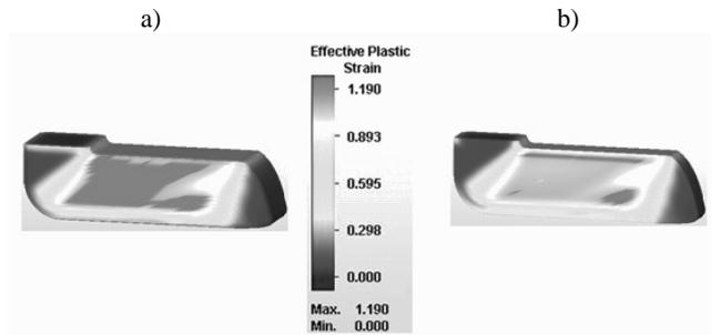
Fig. 4. Comparison of the obtained amount of effective strain and homogeneity of distribution of deformations from the sample edge to its central part, a) at the sample edge, b) at the sample central part
