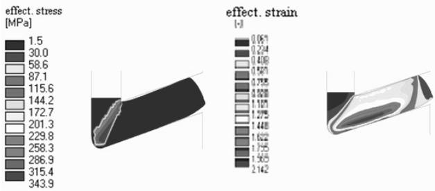
Fig. 3. Development of the effective stress and strain at negative angle  $\phi$
