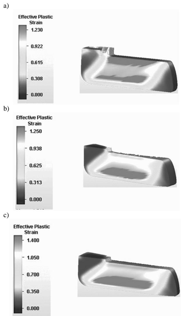
Fig. 5. Development of the effective strain, a) without the channel axle offset, b) with the channel axle offset by  $10^\circ$ , c) with the channel axle offset by  $20^\circ$
