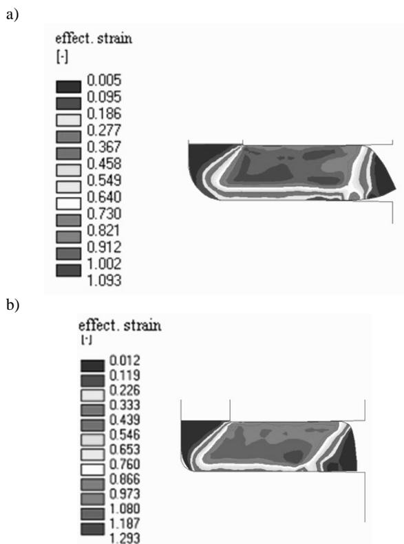
Fig. 2. Development of the effective strain, a) for the channel radii  $R1 = 5.5$  mm,  $R2 = 0.2$  mm, b) for the channel radii  $R1 = 2.4$  mm,  $R2 = 0.2$  mm
