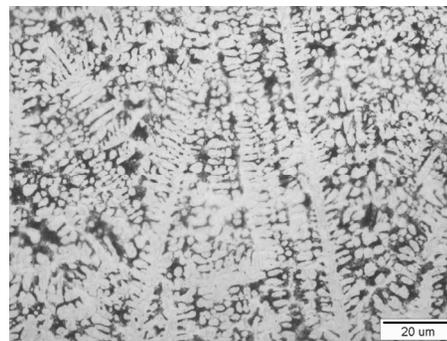
Fig. 1. Central zone of the remelting surface layer of X40CrMoV5-1 steel after alloying with NbC, power range 1.2 kW
