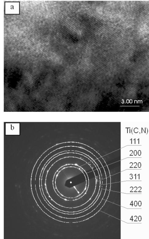
Fig. 5. a) Structure of the thin foil from the TiCN coating deposited onto the hot work tool steel X40CrMoV5-1, b) diffraction pattern from the area as in figure a) and solution of the diffraction pattern
