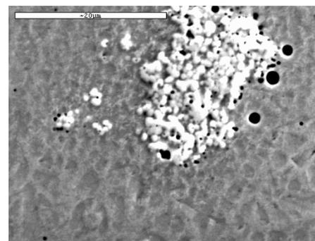
Fig. 2. Surface layer of the X40CrMoV5-1 steel alloyed with the NbC powder, power range 2.0 kW, (SEM)
