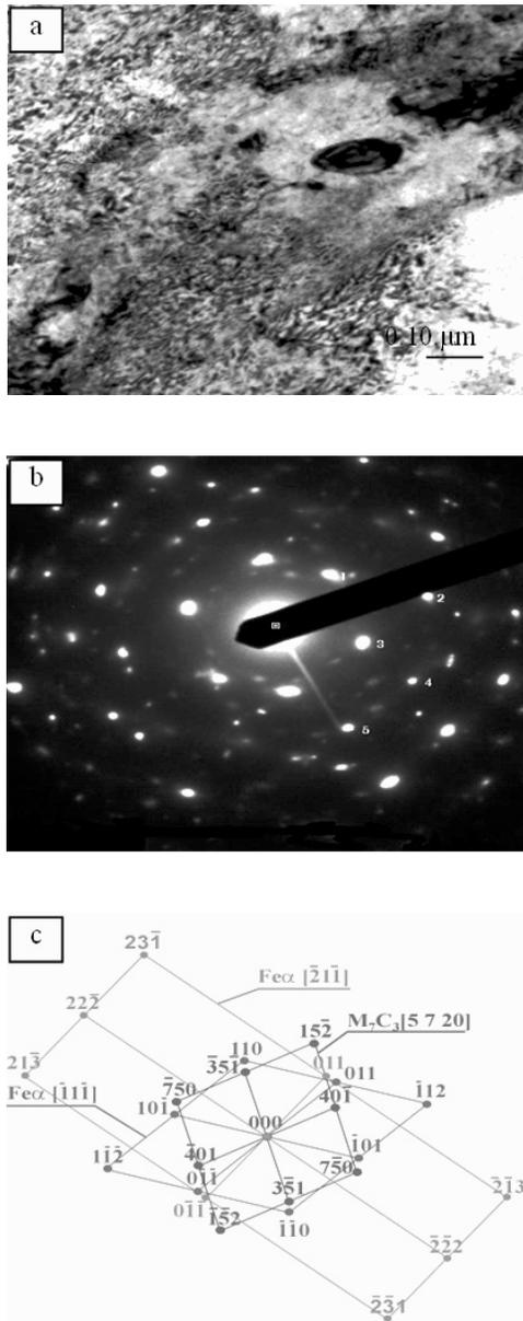
Fig. 4. Structure of the thin foil of X40CrMoV5-1 steel, after alloying NbC, power of bunch laser 1.6 kW: a) a picture in a bright area, a diffraction pattern of area as fig. a), a solution of diffraction pattern from fig. b)
