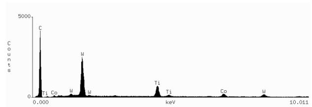
Fig. 3. Results of chemical composition analysis obtained on SEM
