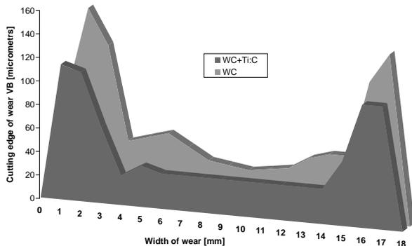
Fig. 6. View of the diminution of the edge after 500 m machining distance
