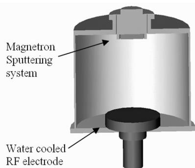
Fig. 1. Schematic of hybrid deposition system
