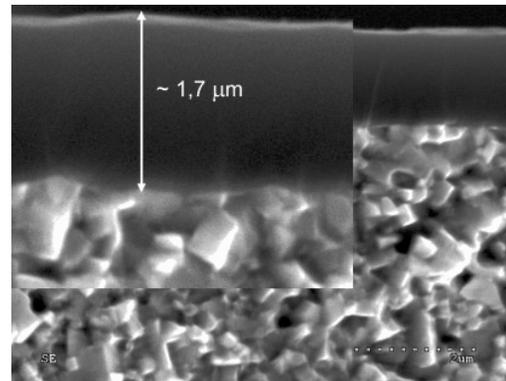
Fig. 2. Fracture of sintered carbide covered with Ti:C layer
