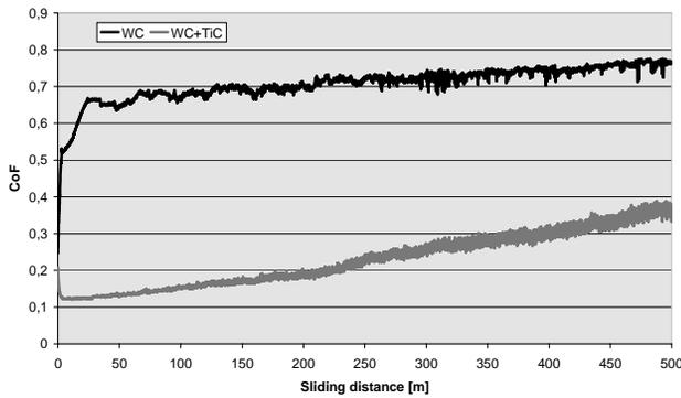
Fig. 4. Friction coefficient investigation results obtained in ball-on-disc method with use of 100Cr6 steel ball, load 10 N
