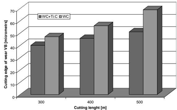
Fig. 7. Diminution rate of the edges after 300, 400 and 500 m machining distance
