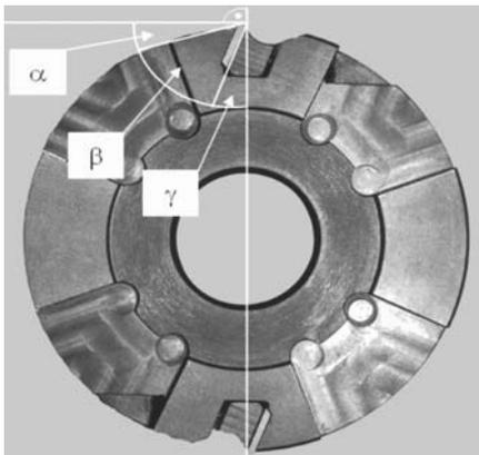
Fig. 5. Picture of the milling cutter heat used in presented investigation
