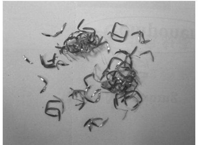
Fig. 6. Continuous chip shape with fine chip breaking
