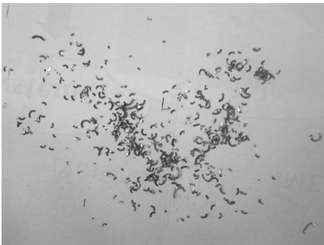
Fig. 5. Discontinuous chip for chatter occurred
