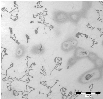
Fig. 3. Microstructure of the alloy AS31-2
