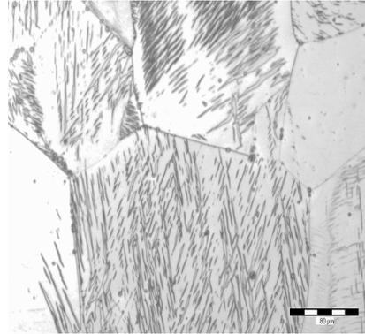
Fig. 5. Microstructure of the alloy Mg-Zr
