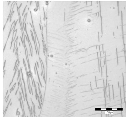
Fig. 6. Microstructure of the alloy Mg-Zr
