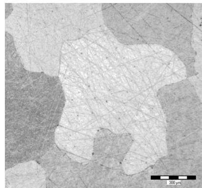
Fig. 7. Structure of pure magnesium
