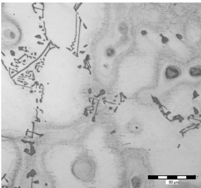
Fig. 4. Microstructure of the alloy AS31-3
