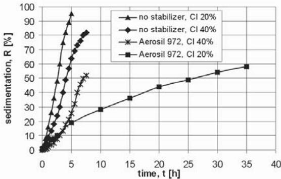
Fig. 5. Sedimentation ratio vs time for MR fluid with different CI content (OKS 600, 7.3 mPa·s)
