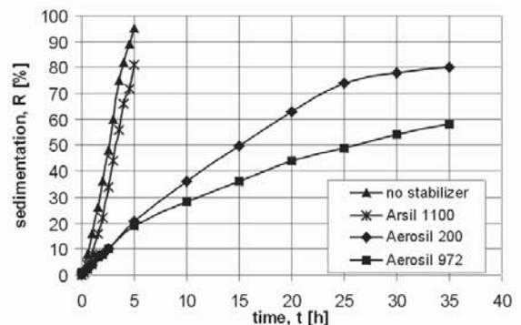
Fig. 4. Sedimentation ratio vs time for MR fluid containing different stabilizer (OKS 600, 7.3 mPa·s, CI 20%)
