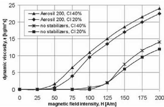
Fig. 2. Dependence of the MR fluid (OKS 1050, 150 mPa·s) dynamic viscosity on the magnetic field intensity
