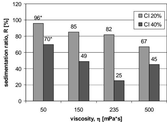
Fig. 3. Sedimentation ratio after 50 h for MR fluids based on OKS 1050 with different viscosity (\* after 10 h)
