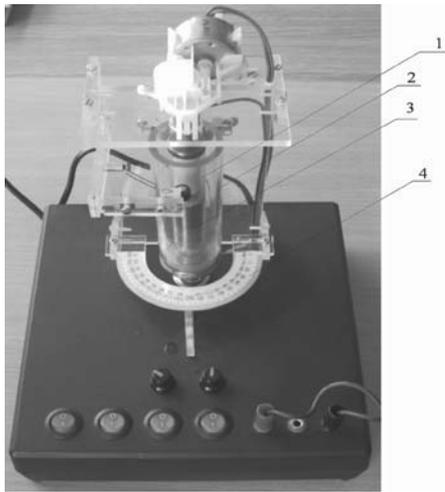
Fig. 1. Apparatus for MR effect measurement. 1 – shaft (drive) and inner cylinder, 2 – outer cylinder, 3 – coil, 4 – needle and angular displacement scale
