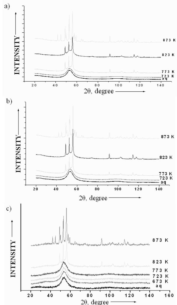
Fig. 1 X-ray diffraction pattern of the  $\text{Co}_{77}\text{Si}_{11.5}\text{B}_{11.5}$  alloy in as quenched state and after annealing in temperature range  $T_a = 723\text{-}873$  K for 30 min.(a), 45 min.(b) and 1 hour (c). The diffractometer's parameters – see Table 1(a).
