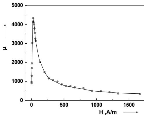
Fig. 4. The maximum permeability  $\mu_{max}$  achieved from the primary curves of magnetization for  $\text{Co}_{77}\text{Si}_{11.5}\text{B}_{11.5}$  alloy in as quenched state
