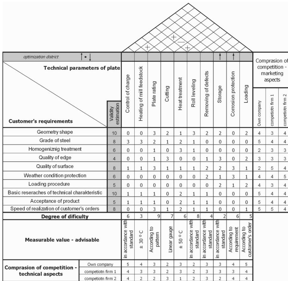
Fig. 3. House of Quality for hot rolling steel
