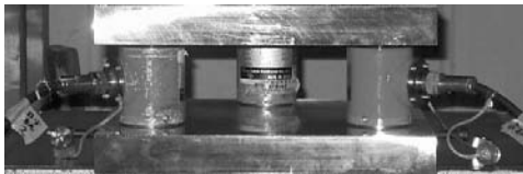
Fig. 1. Three load cells are placed between two sheet steel
