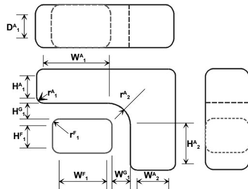
Fig. 2. Basic flat and angled flow chamber
