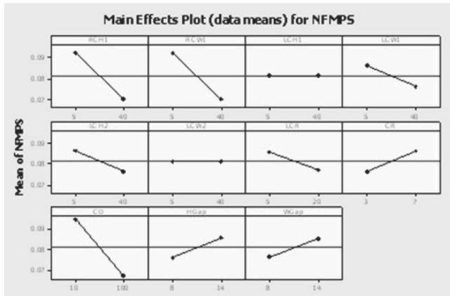
Fig. 7. Main effect of the basic chamber
