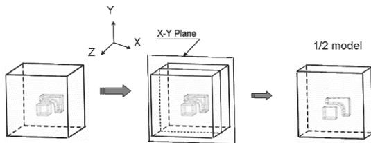
Fig. 3. Simplified for basic chamber
