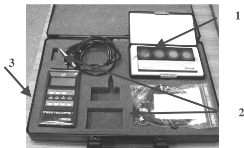
Fig. 6. Complete equipment for measuring the ferrite content, 1. calibration standards, 2. measuring probes, 3. ferritescope.
