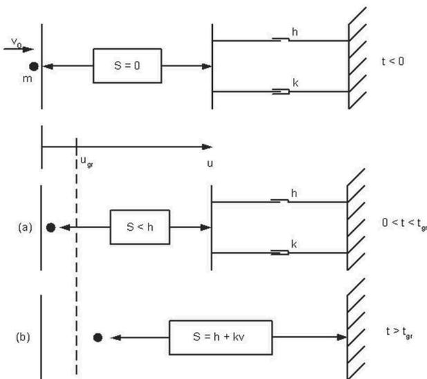
Fig. 1. Diagram of punching process: a) non-destructive deformation phase, b) destructive deformation phase
