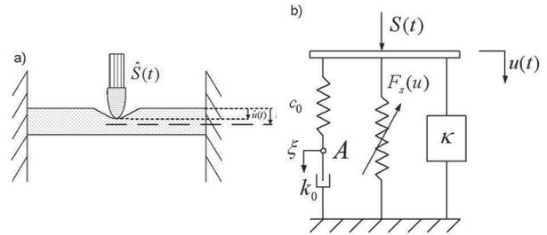
Fig. 3. Diagram of accepted configuration (b) simulating punching process of a material (a) for  $u < u_{gr}$
