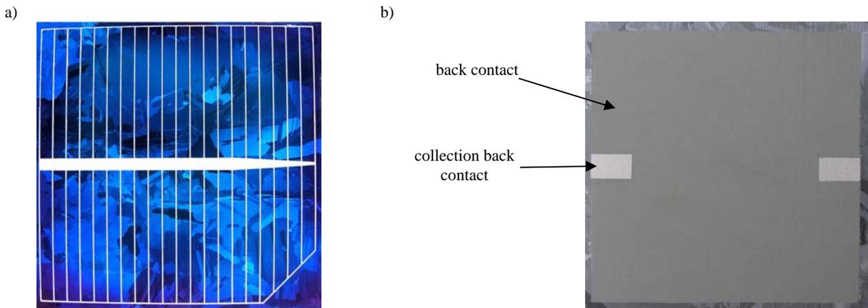
Fig. 10. Metal contacts a) front contact, b) back contact
