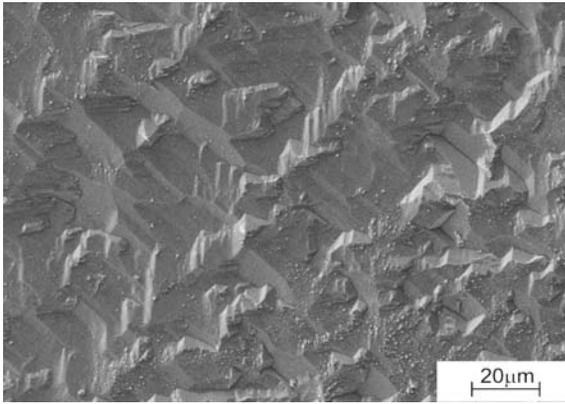
Fig. 3. The topography of silicon wafer surface after saw damage removal
