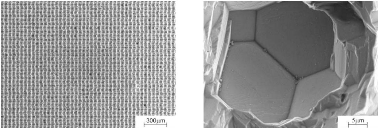
Fig. 6. SEM micrograph of texture corresponding to grid of grooves after removal of distorted layer of thickness 40 μm
