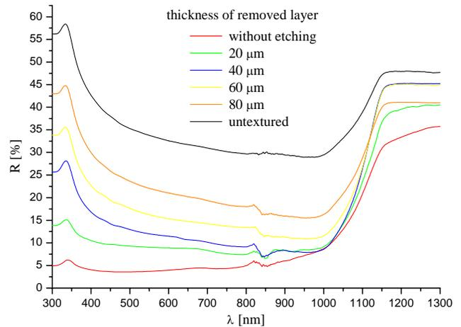
Fig. 9. Reflectance for wafer with texture corresponding to grid of grooves after removal of laser induced damage layer of different thickness
