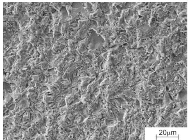
Fig. 2. The topography of silicon wafer surface before saw damage removal
