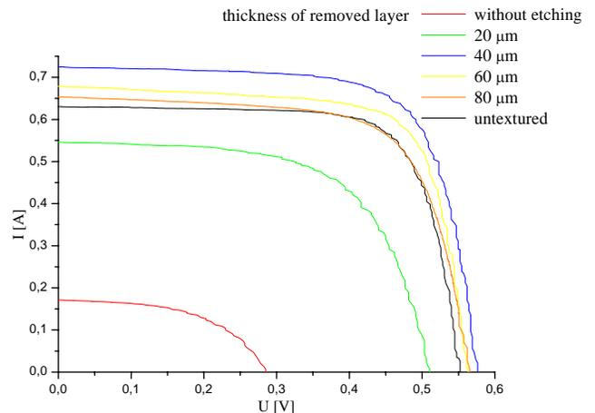
Fig. 11. Current-voltage characteristics of solar cells manufactured from wafers with texture corresponding to parallel grooves after removal of damage induced layer of various thickness
