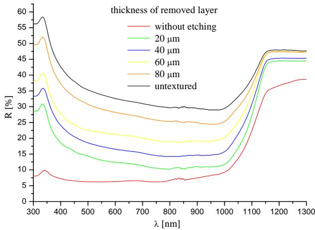
Fig. 8. Reflectance for wafer with texture corresponding to parallel grooves after removal of laser induced damage layer of different thickness
