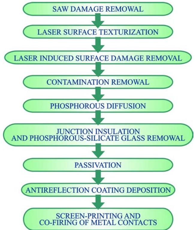
Fig. 1. Technology of multicrystalline silicon solar cells
