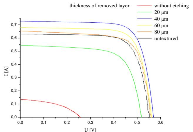
Fig. 12. Current-voltage characteristics of solar cells manufactured from wafers with texture corresponding to grid of grooves after removal of damage induced layer of various thickness
