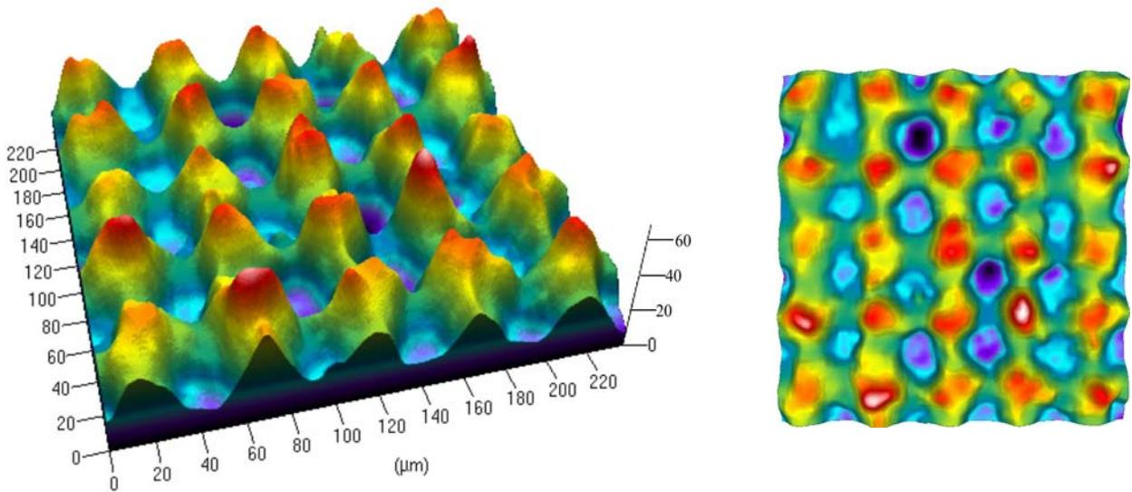
Fig. 5. 3D and 2D confocal laser scanning microscope topographies of texture corresponding to grid of grooves
