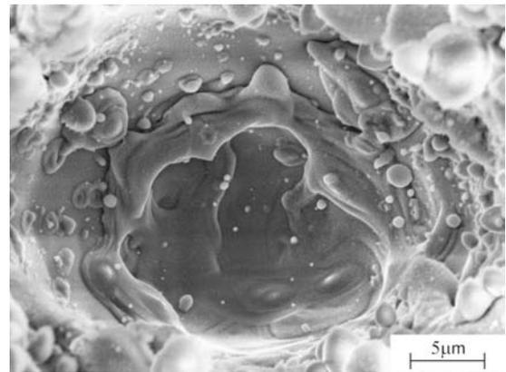
Fig. 4. SEM micrograph of texture corresponding to grid of grooves
