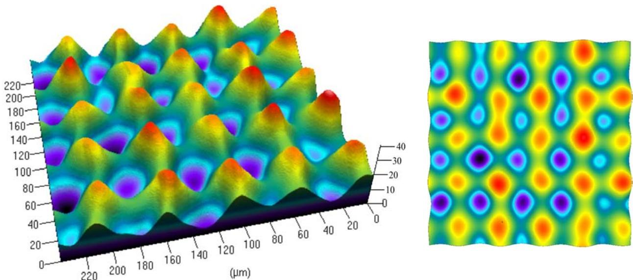
Fig. 7. 3D and 2D confocal laser scanning microscope topographies of texture corresponding to grid of grooves after removal of distorted layer of thickness 40 μm
