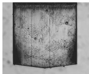
Fig. 2. The wear condition of the punch
