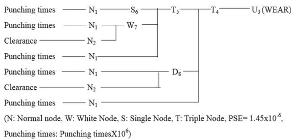
Fig. 4. The relationship between punching parameters and wear of punch's AO-Side
