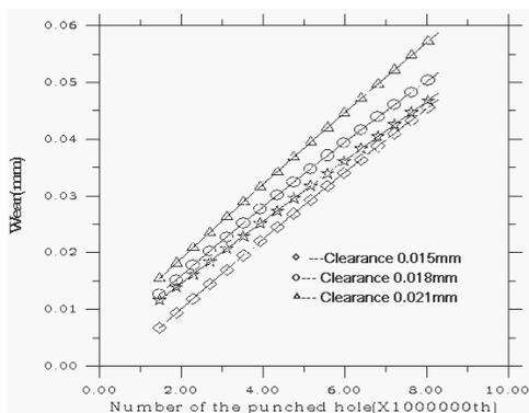
Fig. 5. The relationship between number of the punched hole and wear of punch AO-side
