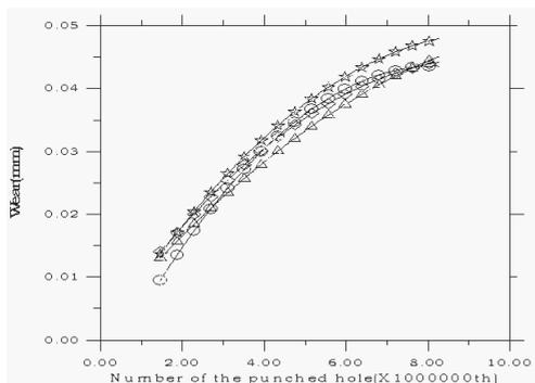
Fig. 6. The relationship between number of the punched hole and wear of punch BO-side
