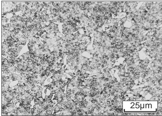
Fig. 6. Structure of X155CrMoV12-1 steel (N=0.085%) after quenching (1020°C/oil) and tempering (2×450°C). Tempered martensite with primary and secondary carbides
