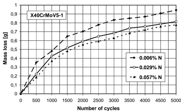
Fig. 13. Relationship of mass loss from number of cycles in wear test for X40CrMoV5-1 steel after quenching (1050°C/oil) and tempering (2x550°C)
