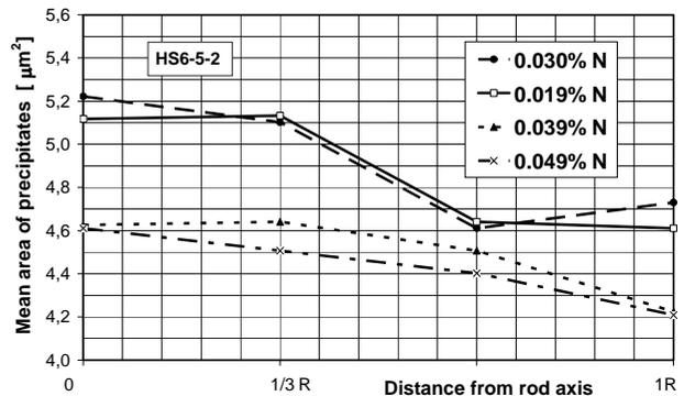
Fig. 10. The influence of concentration of nitrogen and distance from rod axis on the mean area of the precipitates in HS6-5-2 steel after quenching (1220°C/oil) and tempering (2×550°C)
