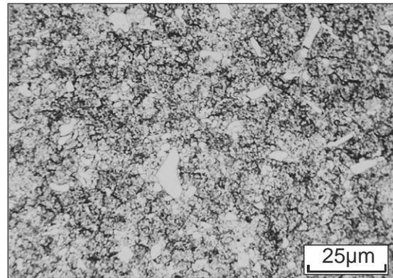
Fig. 1. Structure of X155CrMoV12-1 steel (N=0.085%) in as-annealed condition. Spheroidal and irregular carbides in ferrite
