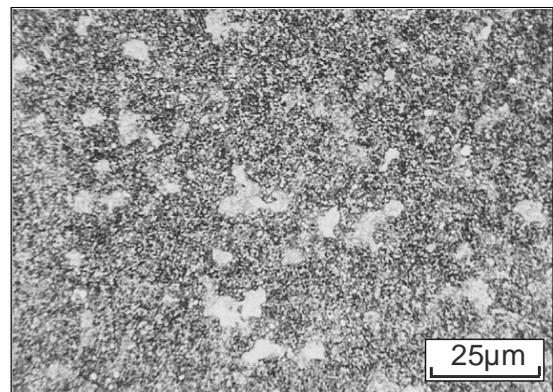
Fig. 2. Structure of HS6-5-2 steel (N=0.057%) in as-annealed condition. Spheroidal and irregular carbides in the ferrite matrix
