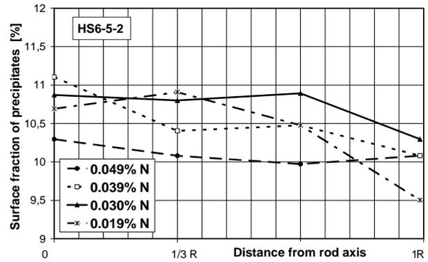
Fig. 9. The influence of concentration of nitrogen and distance from rod axis on the surface fraction of the precipitates in HS6-5-2 steel after quenching (1220°C/oil) and tempering (2×550°C)
