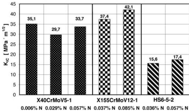
Fig. 15. Collation of values of coefficients  $K_{IC}$  for examined tool steel melts with an increased nitrogen content
