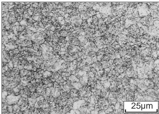
Fig. 8. Structure of X40CrMoV5-1 steel (N=0.057%) after quenching (1050°C/oil) and tempering (2×550°C). Tempered martensite with secondary carbides
