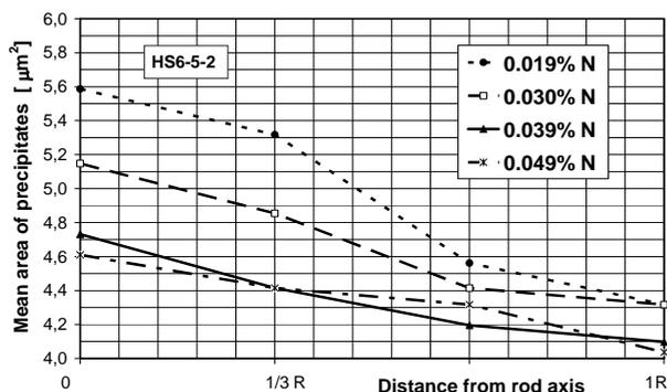
Fig. 5. The influence of concentration of nitrogen and distance from rod axis on the mean area of the precipitates in annealed HS6-5-2 steel
