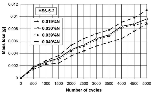
Fig. 12. Relationship of mass loss from number of cycles in wear test for HS6-5-2 steel after quenching (1220°C/oil) and tempering (2x550°C)
