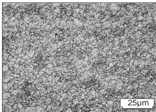
Fig. 3. Structure of X40CrMoV5-1 steel (N=0.057%) in as-annealed condition. Fine-grained ferrite with dispersion carbides
