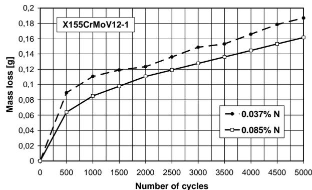
Fig. 14. Relationship of mass loss from number of cycles in wear test for X155CrMoV12-1 steel after quenching (1020°C/oil) and tempering (2x450°C)
