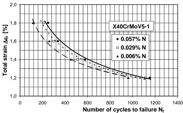
Fig. 16. Collective diagrams of low-cycle fatigue durability at a temperature of 550°C for X40CrMoV5-1 tool steel with diversified nitrogen content
