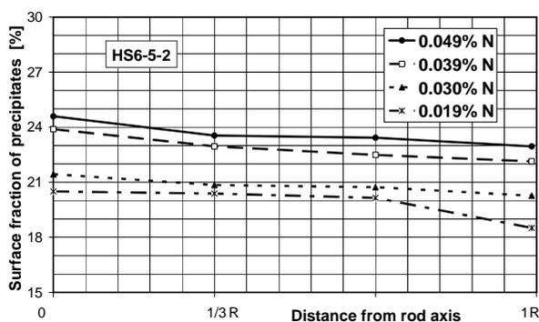
Fig. 4. The influence of concentration of nitrogen and distance from rod axis on the surface fraction of precipitates in annealed HS6-5-2 steel
