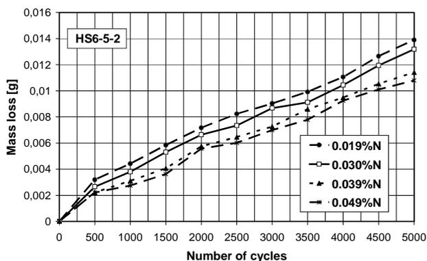
Fig. 11. Relationship of mass loss from number of cycles in wear test for HS6-5-2 steel after quenching (1200°C/oil) and tempering (2x550°C)
