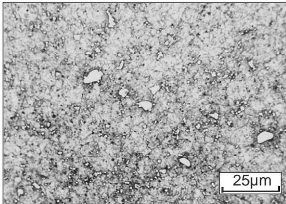
Fig. 7. Structure of HS6-5-2 steel (N=0.057%) after quenching (1220°C/oil) and tempering (2×550°C). Tempered martensite with primary and secondary carbides
