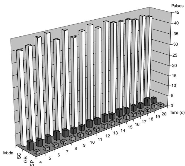
Fig. 8. Pulses for each transference mode in GMAW process; SC: short circuit mode – GB: globular mode; - SP: spray mode
