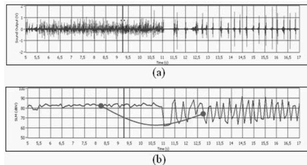
Fig. 4. Oscilogram of short circuit and droplet transfer modes signals
