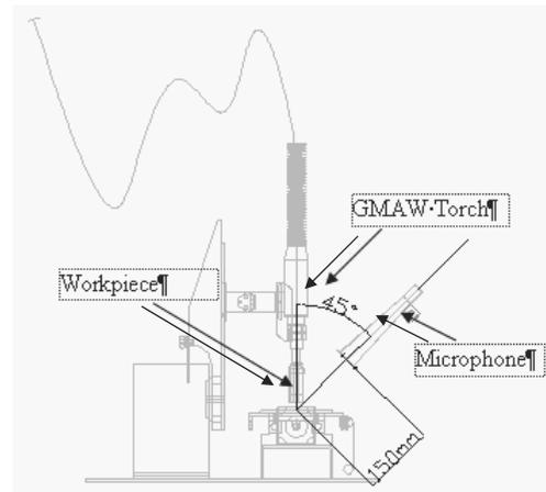
Fig. 2. Microphone positioning
