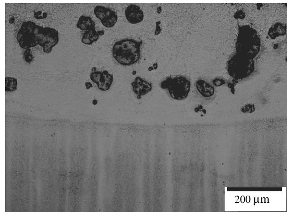
Fig. 14. Microstructure of the WC alloyed sample, X40CrMoV5-1 steel grade, laser power 1.6 kW
