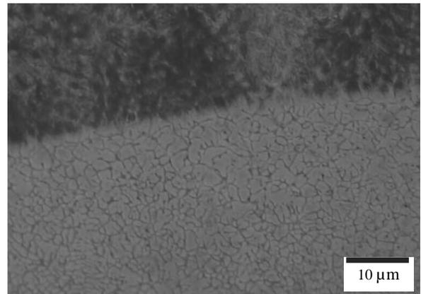
Fig. 13. Microstructures of the VC alloyed sample, 32CrMoV12-28 steel grade, VC powder, laser power 2.0 kW
