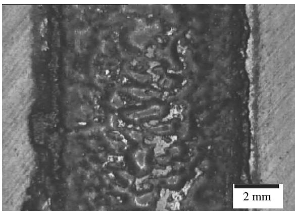
Fig. 5. Structure of the surface layer of the laser remelted samples, 32CrMoV12-28 steel, VC, laser power 2.3 kW
