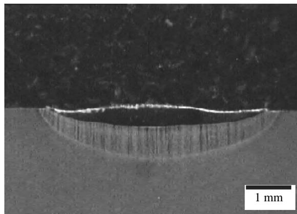
Fig. 7. Shape and thickness of the cross-section of the laser remelted samples, 32CrMoV12-28 steel, VC, laser power 2.0 kW
