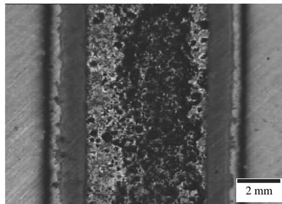
Fig. 9. Structure of the surface layer of the laser remelted samples, WC, laser power 1.2 kW
