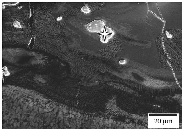
Fig. 16. SEM Microstructure of the 32CrMoV12-28 steel remelted with VC powder, laser power
