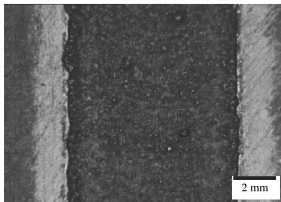
Fig. 8. Structure of the surface layer of the laser remelted samples, 32CrMoV12-28 steel, VC, laser power 1.2 kW
