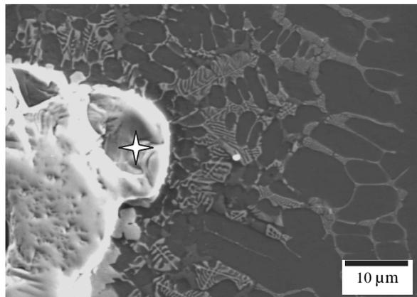
Fig. 17. SEM Microstructure with small eutectics of the X40CrMoV5-1 remelted with WC powder, laser power 1.2 kW
