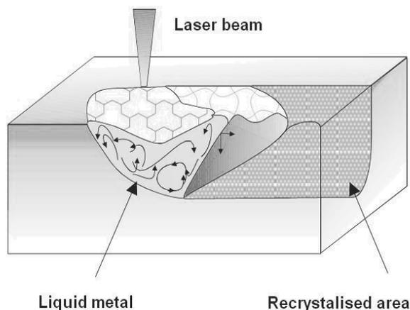
Fig. 1. Theoretical zone view of a cross-section of the laser remelted samples
