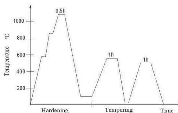
Fig. 2. Heat treatment process carried out for the investigated tool steel
