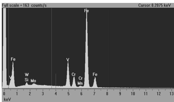
Fig. 21. EDX point analysis made on the marked point in Fig. 18
