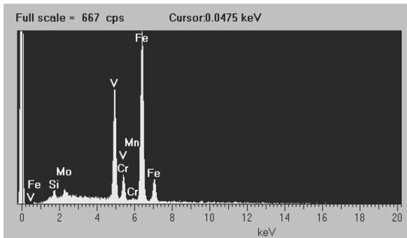
Fig. 19. EDX point analysis made on the marked point in Fig. 16
