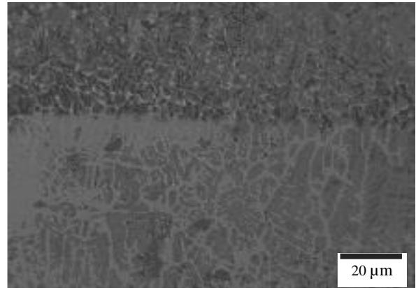
Fig. 12. Microstructures of the WC alloyed sample, 32CrMoV12-28 steel grade, WC powder, laser power 2.0 kW
