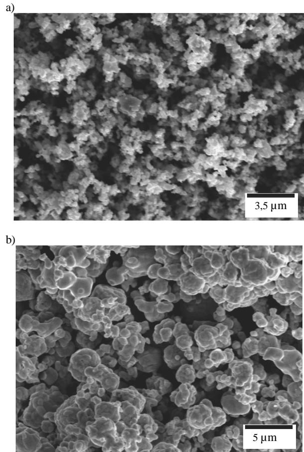
Fig. 4. Ceramic carbide powders used for alloying, a) Vanadium carbide VC, b) Tungsten carbide WC (SEM)
