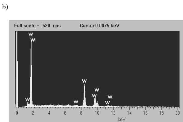
Fig. 15. a) SEM Microstructure of the of the 32CrMoV12-28 steel remelted with WC powder, b) EDX point analysis made on the marked point in a)
