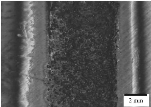
Fig. 10. Structure of the surface layer of the laser remelted samples WC, laser power 2.3 kW
