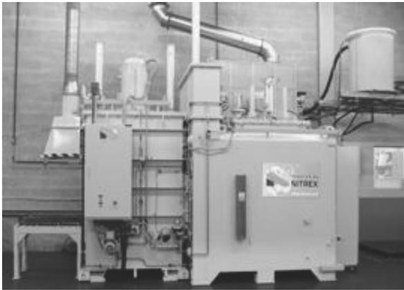
Fig. 3. Nitrex Metal Inc horizontal chamber furnace
