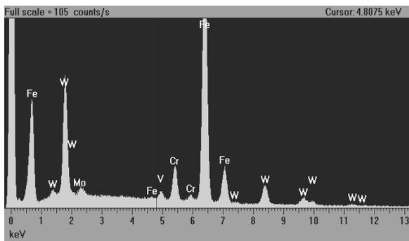
Fig. 20. EDX point analysis made on the marked point in Fig. 17
