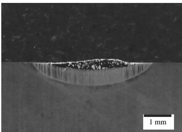
Fig. 6. Shape and thickness of the cross-section of the laser remelted samples, 32CrMoV12-28 steel, WC, laser power 2.0 kW
