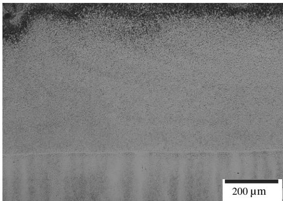
Fig. 11. Microstructure of the VC alloyed sample, X40CrMoV5-1 steel grade, laser power 2.3 kW
