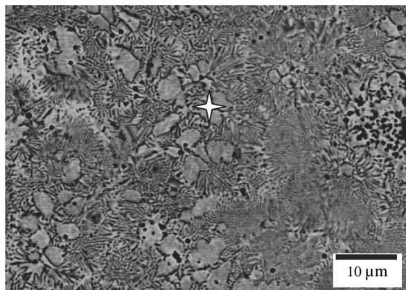
Fig. 18. SEM Microstructure of the X40CrMoV5-1 remelted with VC powder, laser power 1.6 kW
