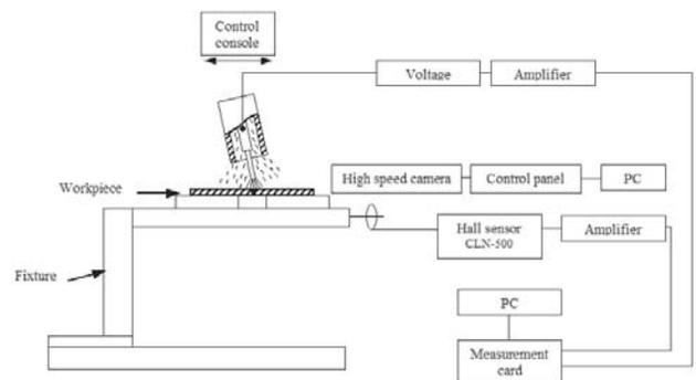
Fig. 1. Experimental platform
