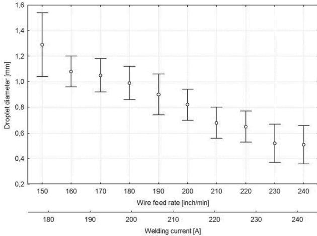
Fig. 2. Influence of wire speed rate (welding current) on droplet diameter
