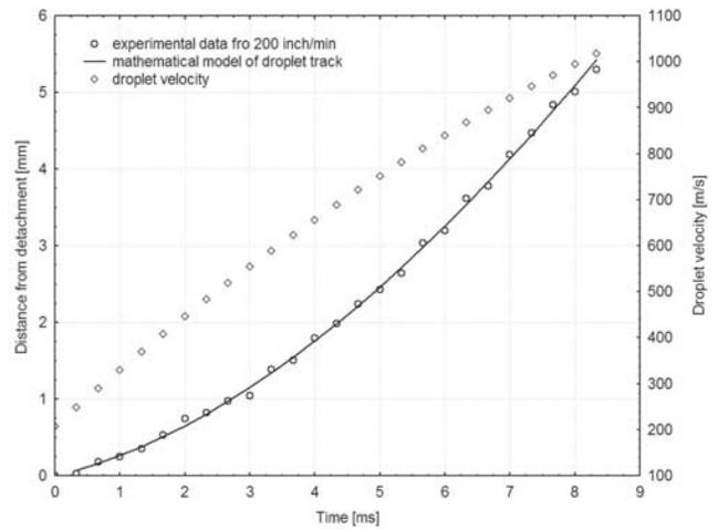
Fig. 3. The droplet flight trajectory and droplet velocity for wire feed speed 200 inch/min, comparison experimental data with mathematical model based on formula 2 and 4
