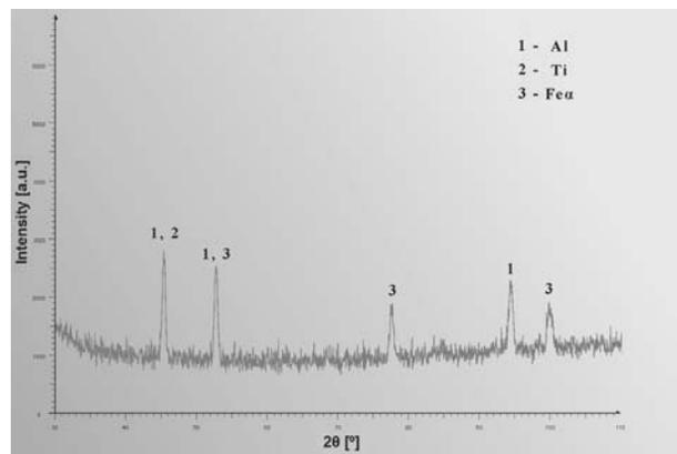
Fig. 1. The X-ray diffraction patterns of  $Al_{67}Ti_{25}Fe_8$  powder alloy after 10 hrs of mechanical alloying
