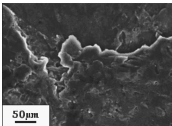
Fig. 8. Structure of powder particle surface of  $Al_{67}Ti_{25}Fe_8$  alloy after 100 hrs of mechanical alloying
