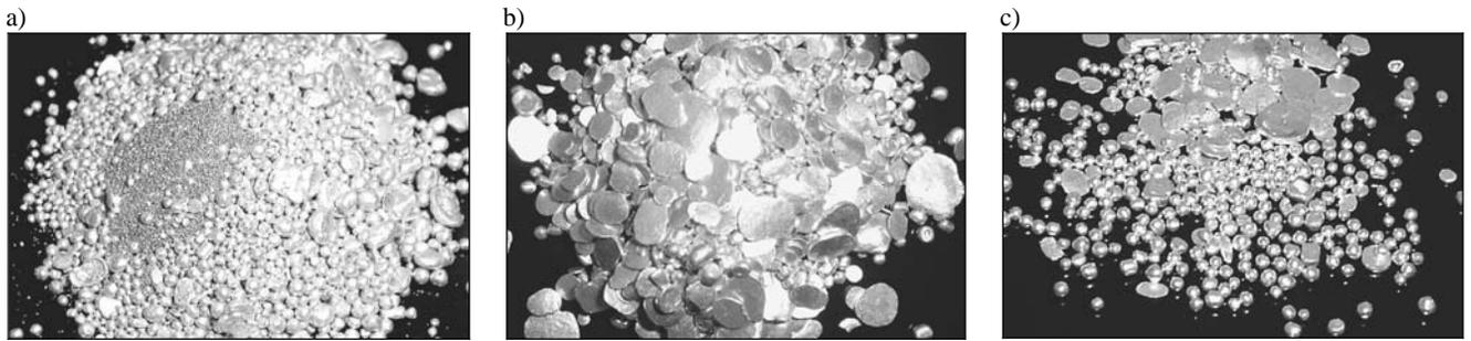
Fig. 3. Powder particles after a) 10hrs, b) 45hrs, c) 100hrs, of mechanical alloying (macroscopic observation)
