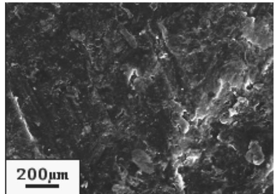
Fig. 6. Structure of powder particle surface of  $\text{Al}_{67}\text{Ti}_{25}\text{Fe}_8$  alloy after 10 hrs of mechanical alloying
