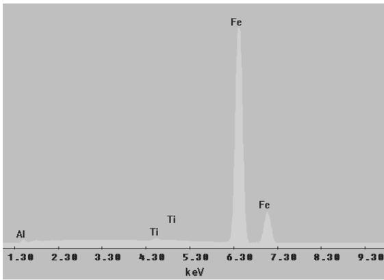
Fig. 14. Plot of the X-ray dispersive energy spectrometer measurement from the  $Al_{67}Ti_{25}Fe_8$  alloy after 100hrs of mechanical alloying process (point 1 in Fig. 15.)
