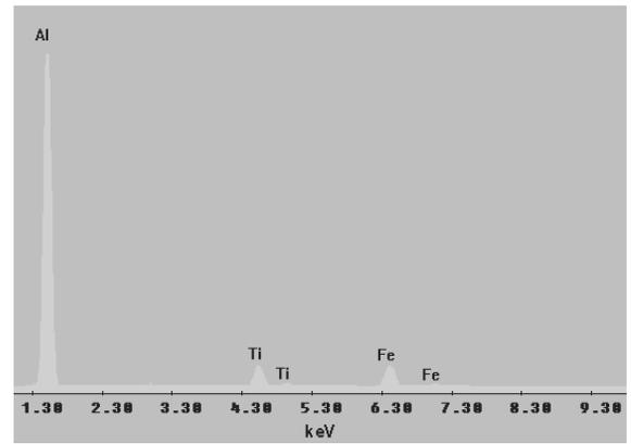
Fig. 17. Plot of the X-ray dispersive energy spectrometer measurement from the  $Al_{67}Ti_{25}Fe_8$  alloy after 100hrs of mechanical alloying process (point 4 in Fig. 15.)
