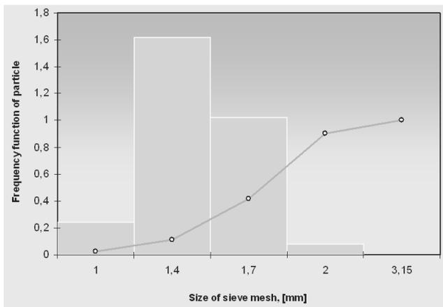
Fig. 20. Particle size distribution of studied  $\text{Al}_{67}\text{Ti}_{25}\text{Fe}_8$  powder after 100hrs. of mechanical alloying
