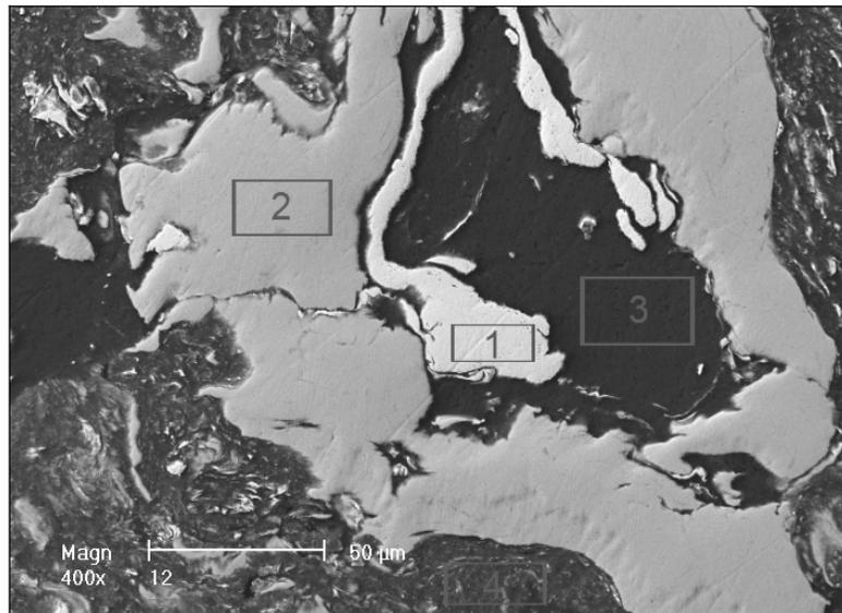
Fig. 13. Cross section of  $\text{Al}_{67}\text{Ti}_{25}\text{Fe}_8$  powder alloy mechanically milled for 100 hrs (SEM)
