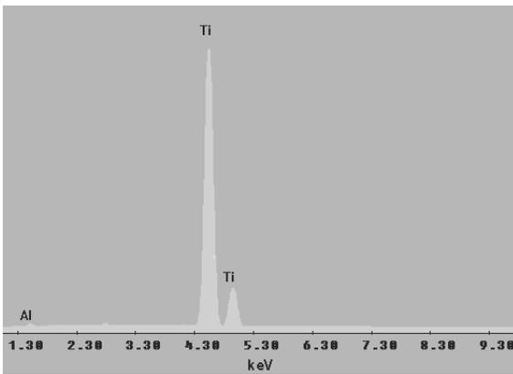
Fig. 15. Plot of the X-ray dispersive energy spectrometer measurement from the  $Al_{67}Ti_{25}Fe_8$  alloy after 100hrs of mechanical alloying process (point 2 in Fig. 15.)
