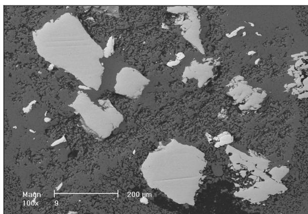
Fig. 9. Cross section of particles of  $Al_{67}Ti_{25}Fe_8$  initial powder alloy (SEM)
