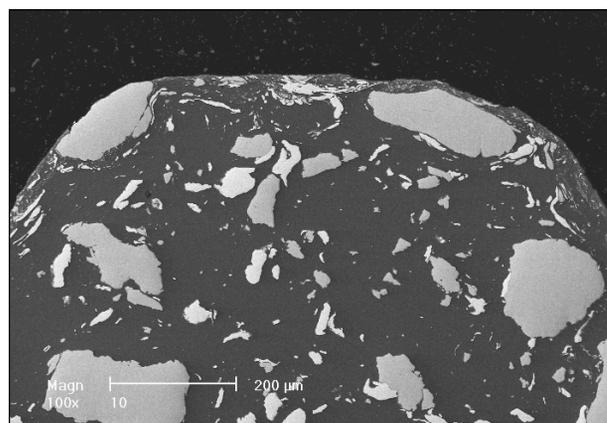
Fig. 10. Cross section of particles of  $Al_{67}Ti_{25}Fe_8$  powder alloy mechanically milled for 10 hrs (SEM)
