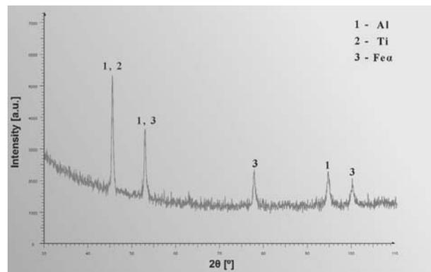
Fig. 2. The X-ray diffraction patterns of  $Al_{67}Ti_{25}Fe_8$  powder alloy after 100 hrs of mechanical alloying
