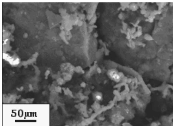
Fig. 7. Structure of powder mixture of  $Al_{67}Ti_{25}Fe_8$  alloy after 45hrs of mechanical alloying
