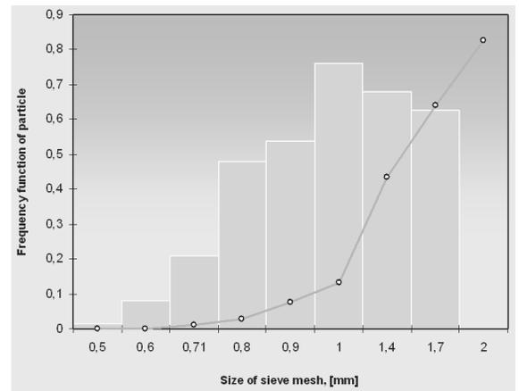
Fig. 18. Particle size distribution of studied  $Al_{67}Ti_{25}Fe_8$  powder after 10hrs. of mechanical alloying
