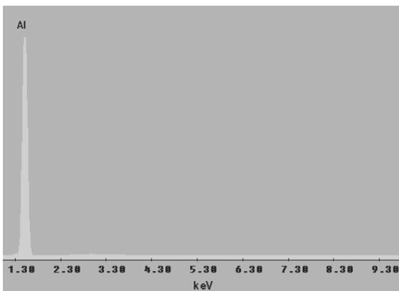
Fig. 16. Plot of the X-ray dispersive energy spectrometer measurement from the  $Al_{67}Ti_{25}Fe_8$  alloy after 100hrs of mechanical alloying process (point 3 in Fig. 15.)
