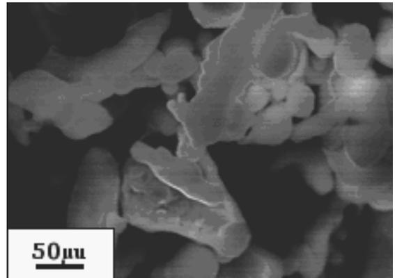
Fig. 5. Structure of initial powder mixture of  $\text{Al}_{67}\text{Ti}_{25}\text{Fe}_8$  alloy
