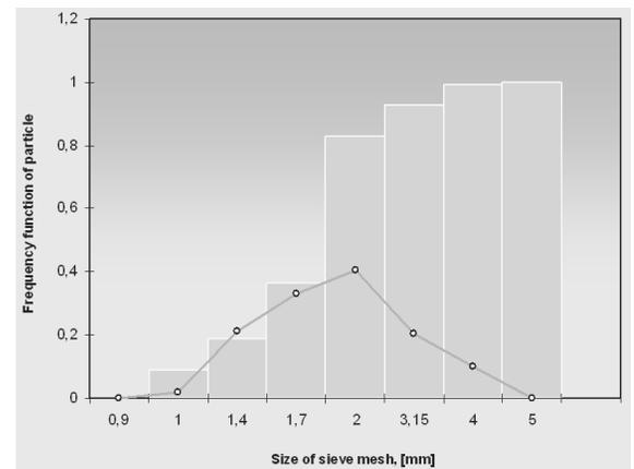
Fig. 19. Particle size distribution of studied  $Al_{67}Ti_{25}Fe_8$  powder after 45hrs. of mechanical alloying
