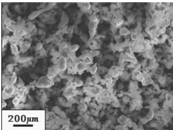
Fig. 4. Structure of initial powder mixture of  $\text{Al}_{67}\text{Ti}_{25}\text{Fe}_8$  alloy
