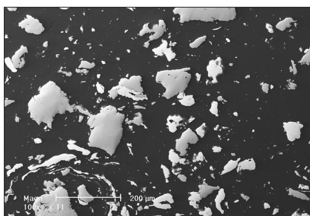
Fig. 11. Cross section of particles of  $Al_{67}Ti_{25}Fe_8$  powder alloy mechanically milled for 45 hrs (SEM)
