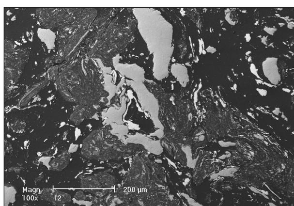
Fig. 12. Cross section of particles of  $Al_{67}Ti_{25}Fe_8$  powder alloy mechanically milled for 100 hrs (SEM)
