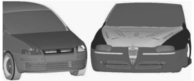
Fig. 15. Vehicle FEM model
