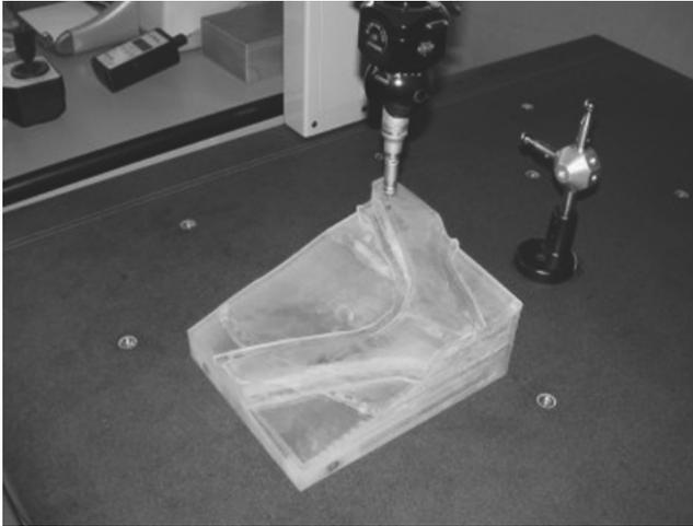
Fig. 14. Prototyped tile under measurement machine
