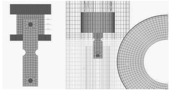
Fig. 7. Lower leg knee joint FEM model
