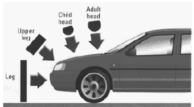
Fig. 4. Pedestrian tests according to WG17 - EuroNCAP
