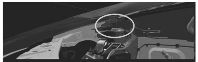
Fig. 13. Distance between dome and bonnet frame
