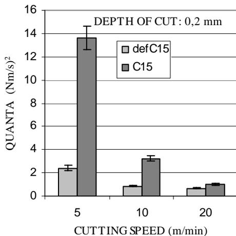
Fig. 5. Relation between energy quanta and cutting speed of normalized (C15) and cold deformed (defC15) steels with depth of cut  $a_1 = 0.2$  mm
