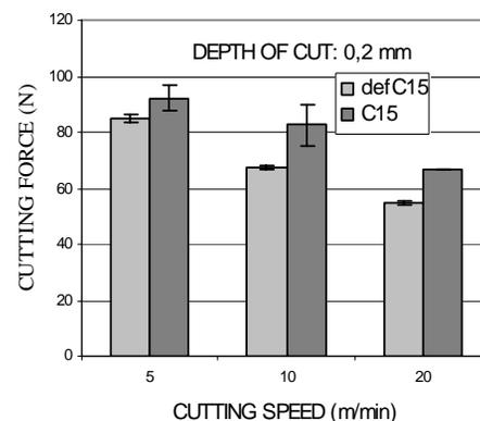
Fig. 3. Magnitude of the cutting force for normalized (C15) and cold deformed (defC15) steels with different cutting speed and depth of cut  $a_1 = 0.2$  mm
