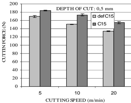
Fig. 4. Magnitude of the cutting force of normalized (C15) and cold deformed (defC15) steels with different cutting speed and depth of cut  $a_2 = 0.5$  mm
