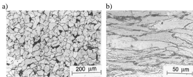
Fig.1. Microstructures of work materials: a) C15 normalized and b) def C15 cold deformed
