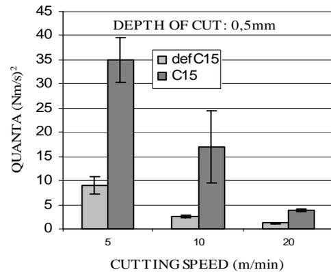
Fig. 6. Relation between energy quanta and cutting speed of normalized (C15) and cold deformed (defC15) steels with depth of cut  $a_2 = 0.5$  mm
