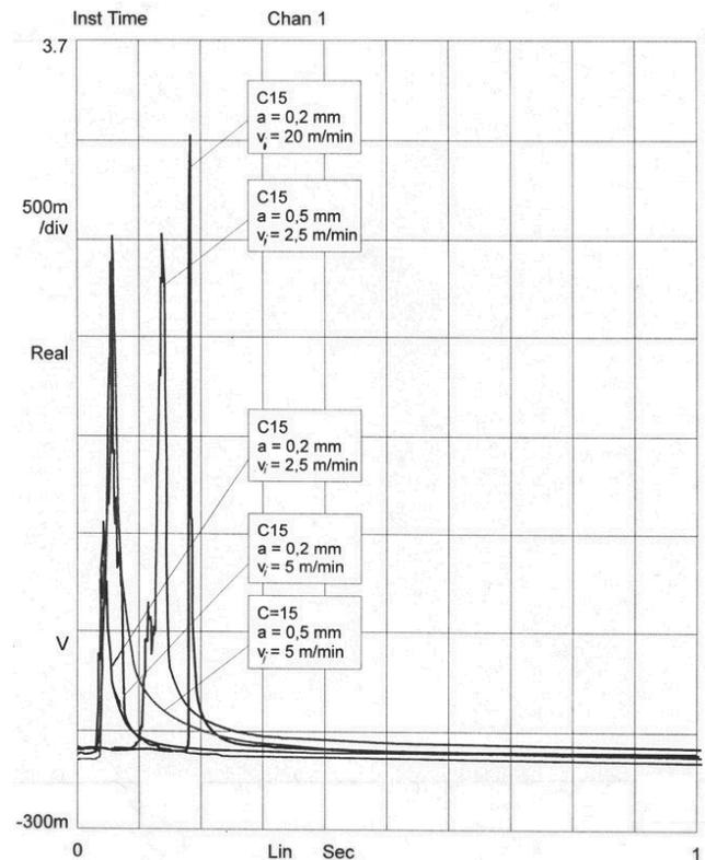
Fig. 7. Signals of thermal potential in cutting normalized C15 and cold deformed steel C15def
