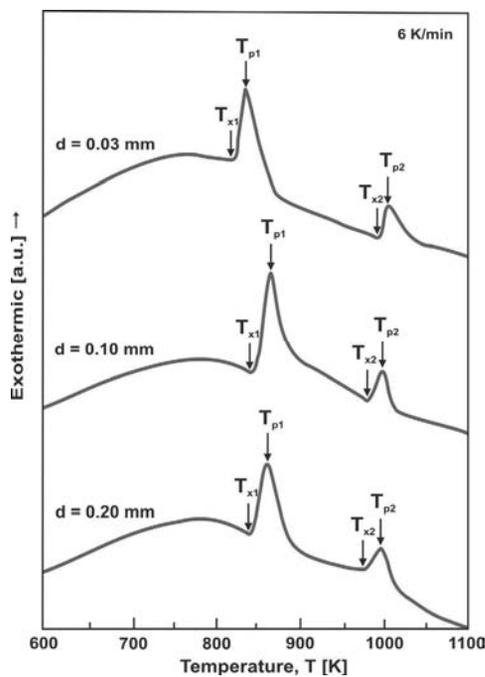
Fig. 7. DTA curves of  $\text{Fe}_{36}\text{Co}_{36}\text{B}_{19}\text{Si}_5\text{Nb}_4$  glassy alloy ribbons in as-cast state
