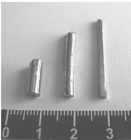
Fig. 1. Outer morphology of cast glassy  $\text{Fe}_{36}\text{Co}_{36}\text{B}_{19}\text{Si}_5\text{Nb}_4$  alloy rods with diameters of 2, 3 and 4 mm
