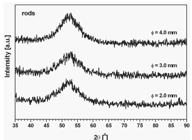
Fig. 5. X-ray diffraction patterns of  $\text{Fe}_{36}\text{Co}_{36}\text{B}_{19}\text{Si}_5\text{Nb}_4$  glassy rods in as-cast state with diameter of 2, 3 and 4 mm
