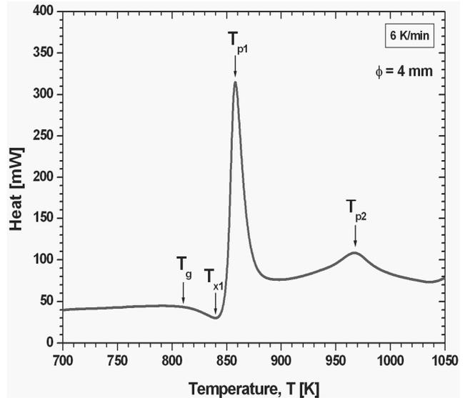
Fig. 10. DSC curve of  $\text{Fe}_{36}\text{Co}_{36}\text{B}_{19}\text{Si}_5\text{Nb}_4$  glassy alloy rod in as-cast state with diameter of 4 mm
