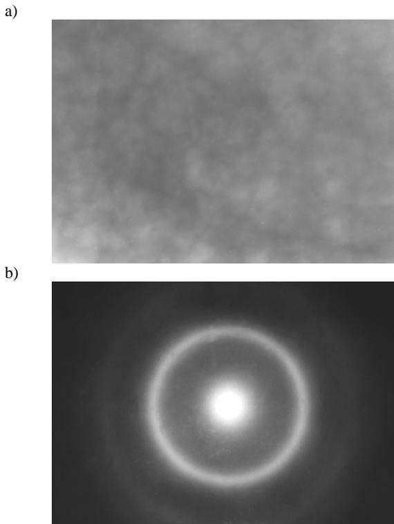
Fig. 6. Transmission electron micrograph, 66 000x (a) and electron diffraction pattern (b) of the as-cast glassy  $\text{Fe}_{36}\text{Co}_{36}\text{B}_{19}\text{Si}_5\text{Nb}_4$  rod with a diameter of 4 mm
