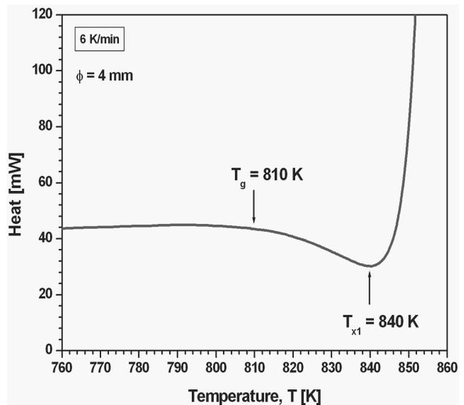
Fig. 11. Glass transition temperature ( $T_g$ ) and onset crystallization temperature ( $T_{x1}$ ) of tested glassy rod in as-cast state
