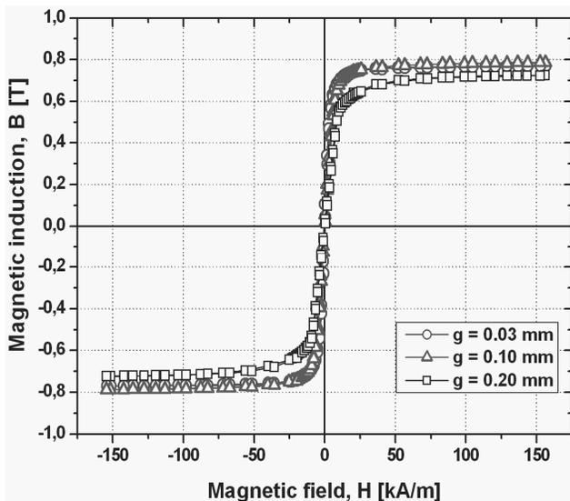
Fig. 9. Hysteresis loops of tasted  $\text{Fe}_{36}\text{Co}_{36}\text{B}_{19}\text{Si}_5\text{Nb}_4$  glassy alloy ribbons
