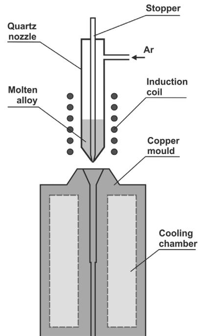
Fig. 2. Schematic illustration of the pressure die casting equipment used for casting bulk amorphous samples
