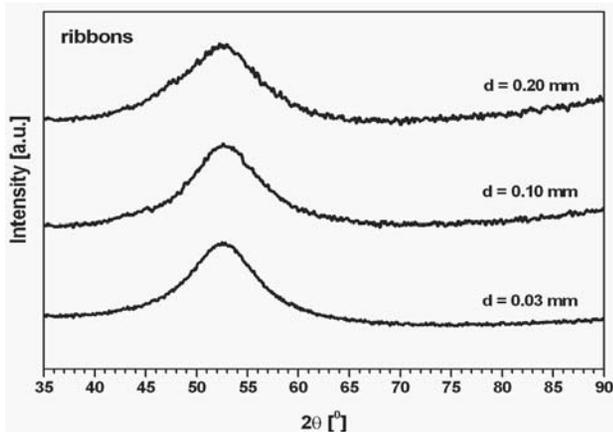
Fig. 3. X-ray diffraction patterns of  $\text{Fe}_{36}\text{Co}_{36}\text{B}_{19}\text{Si}_5\text{Nb}_4$  glassy ribbons in as-cast state with thickness of 0.03, 0.10 and 0.20 mm
