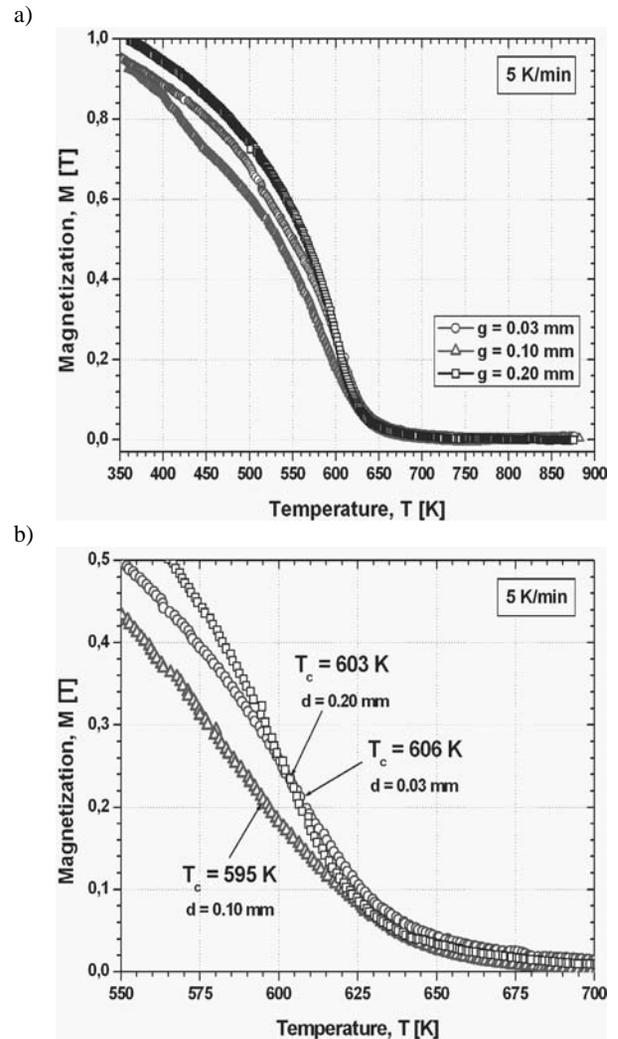
Fig. 8. Normalized curves of magnetization of  $\text{Fe}_{36}\text{Co}_{36}\text{B}_{19}\text{Si}_5\text{Nb}_4$  glassy alloy in form of ribbons in as-cast state (a), Curie temperatures of cast glassy  $\text{Fe}_{36}\text{Co}_{36}\text{B}_{19}\text{Si}_5\text{Nb}_4$  alloy ribbons (b)
