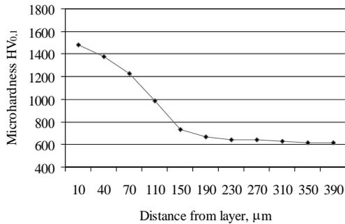
Fig. 5. Microhardness changes in the nitriding layer of the plasma nitrided hot work steel X37CrMoV5-1 type
