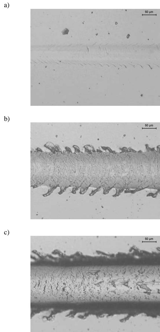
Fig. 4. Scratches with critical load: a)  $Lc_3$ -flaking on the scratch edge, b)  $Lc_4$ -partial delamination, c)  $Lc_5$ -total delamination; CrN coating deposited onto heat treated X37CrMoV5-1 steel substrate
