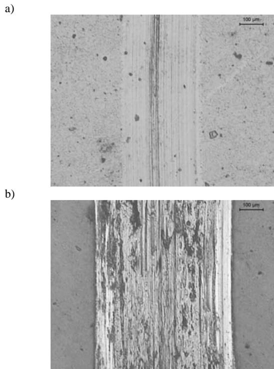
Fig. 9. Microphotography of wear track on the surface of investigated samples for CrN coating onto plasma nitrided X37CrMoV5-1 steel type: a) 20°C, b) 500°C; 7500 revolutions
