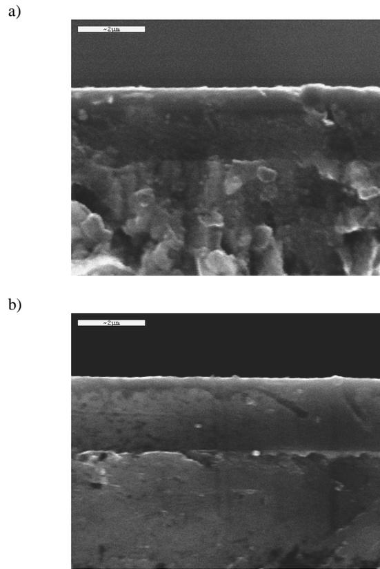
Fig. 2. Fracture of the CrN coatings deposited onto hot work steel X37CrMoV5-1 type: a) after heat treated, b) after plasma nitrited
