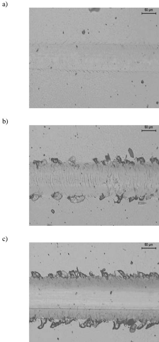
Fig. 3. Scratches with critical load: a)  $Lc_3$ -flaking on the scratch edge, b)  $Lc_4$ -partial delamination, c)  $Lc_5$ -total delamination; CrN coating deposited onto plasma nitrided X37CrMoV5-1 steel substrate
