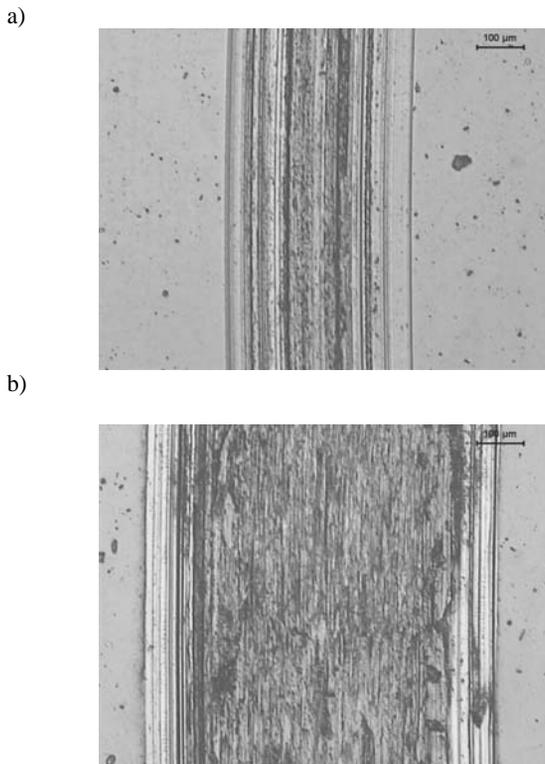
Fig. 8. Microphotography of wear track on the surface of investigated samples for CrN coating onto heat treated X37CrMoV5-1 steel type: a) 20°C, b) 500°C; 7500 revolutions
