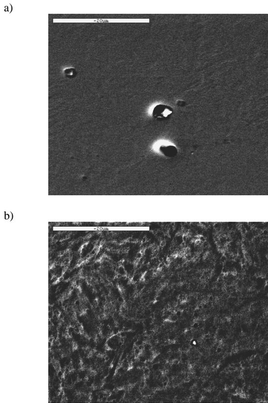
Fig. 1. Topography of the CrN coatings deposited onto hot work steel X37CrMoV5-1 type: a) after heat treated, b) after plasma nitrited
