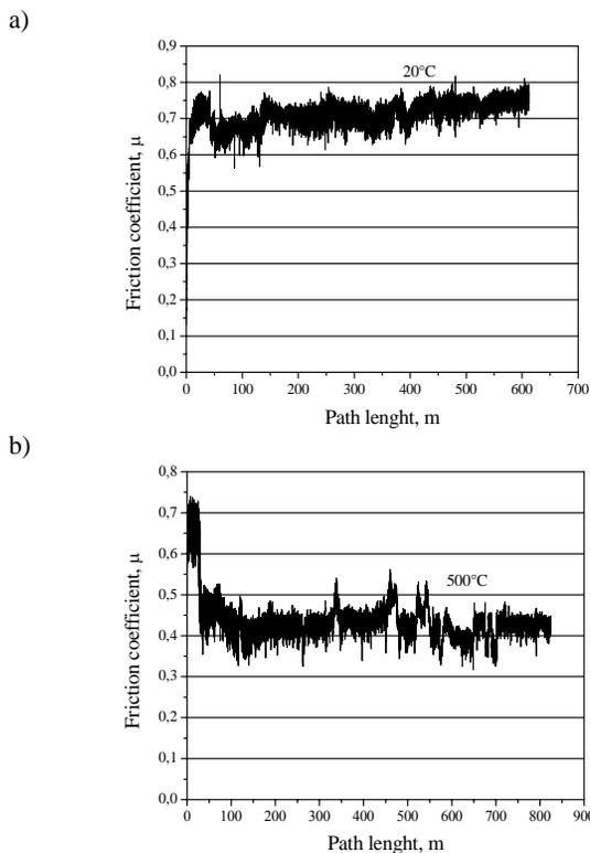
Fig. 6. Friction coefficient changes versus wear path length for CrN coating onto heat treated X37CrMoV5-1 steel type: a) 20°C, b) 500°C; 7500 revolutions
