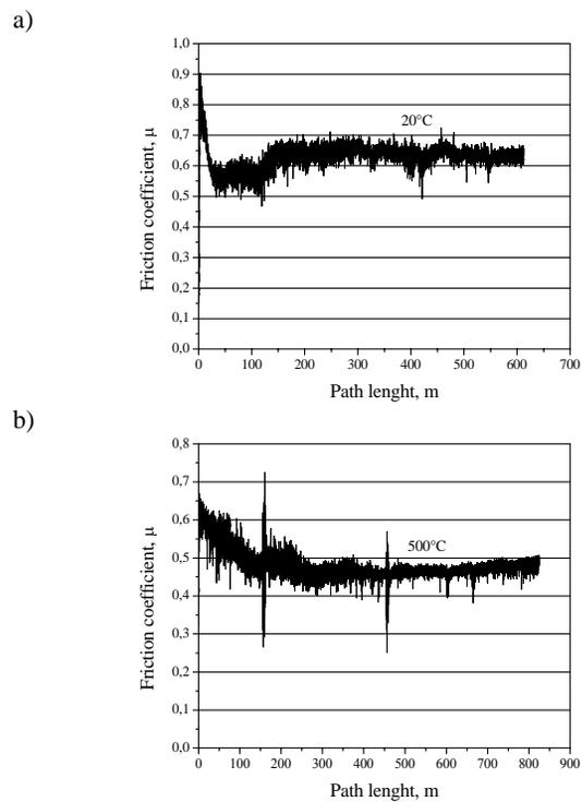
Fig. 7. Friction coefficient changes versus wear path length for CrN coating onto plasma nitrided X37CrMoV5-1 steel type: a) 20°C, b) 500°C; 7500 revolutions
