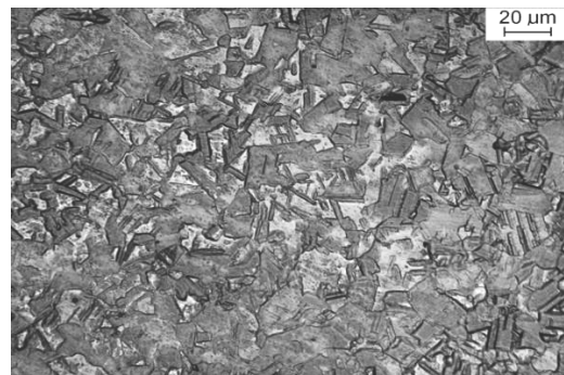
Fig. 4. Austenitic structure of the 26Mn-3Si-3Al-Nb-Ti steel after solution heat treatment from a temperature of 900°C
