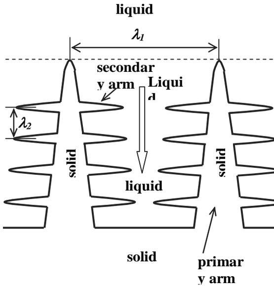
Fig. 2. Interdendritic channels in columnar dendritic mushy zone showing a liquid flow parallel to primary dendrite arms
