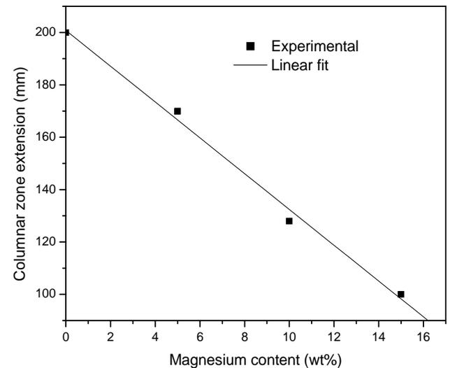
Fig. 3. Extension of columnar zone as function of magnesium content
