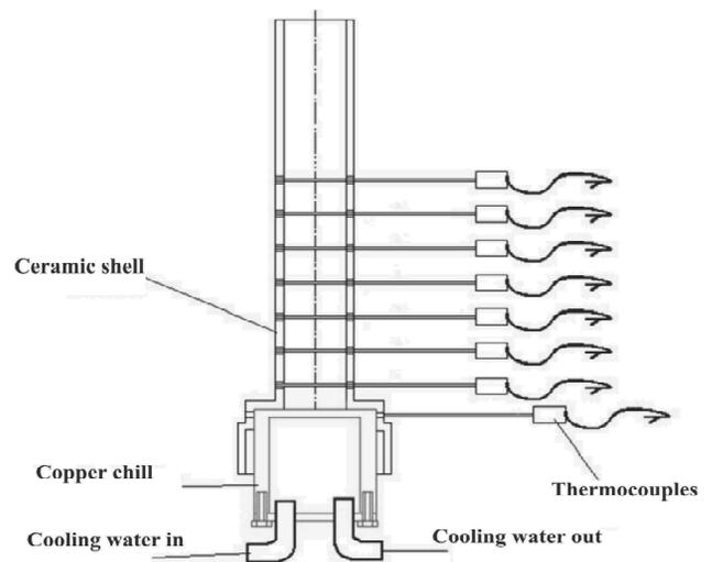
Fig. 1. Schematic representation of the experimental device used to promote unidirectional solidification
