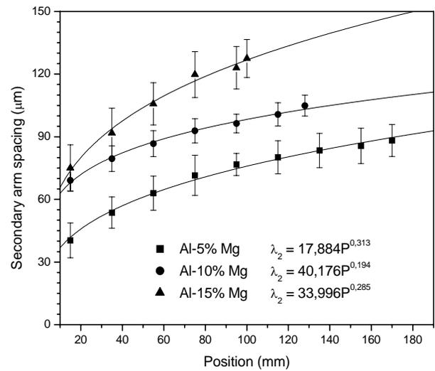
Fig. 5. Variation of secondary dendrite arm spacing as function of the distance from metal/mold interface during solidification of Al-Mg alloys containing 5, 10 and 15 wt% magnesium
