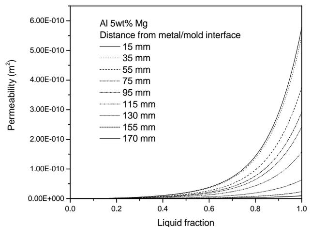
Fig. 6. Variation of permeability of interdendritic channels as function of liquid fraction at different distances from metal/mold interface for the alloy Al 5 wt% Mg
