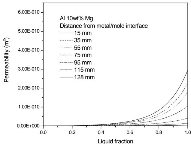
Fig. 7. Variation of permeability of interdendritic channels as function of liquid fraction at different distances from metal/mold interface for the alloy Al 10 wt% Mg
