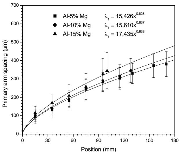
Fig. 4. Variation of primary dendrite arm spacing as function of the distance from metal/mold interface during solidification of Al-Mg alloys containing 5, 10 and 15 wt% magnesium
