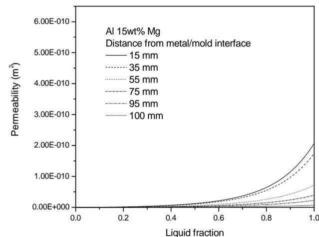
Fig. 8. Variation of permeability of interdendritic channels as function of liquid fraction at different distances from metal/mold interface for the alloy Al 15 wt% Mg
