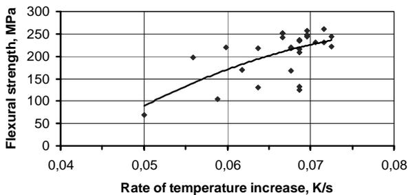
Fig. 10. Relation between flexural strength and rate of temperature increase
