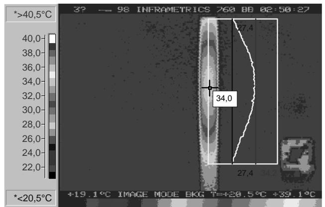
Fig. 4. Thermographic image of sample aged 1992 hours in 200 °C captured 165 seconds after the end of heating
