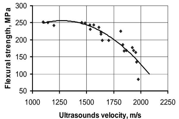
Fig. 15. Experimental relation between flexural strength and ultrasounds velocity
