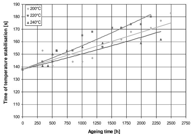
Fig. 7. Relationship between ageing time and the time of temperature stabilization
