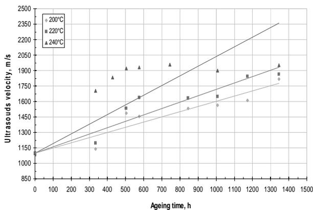
Fig. 12. Dependence of ultrasound wave propagation velocity on ageing time and temperature
