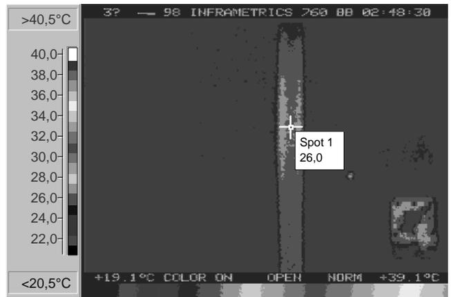
Fig. 3. Thermographic image of sample aged 1992 hours in 200 °C captured 30 seconds after the end of heating
