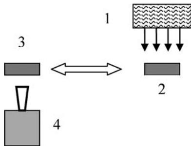
Fig. 2. Thermovision test stand: 1 – IR heater, 2 – the sample in heating position, 3 – the sample in temperature scanning position, 4- thermovision camera
