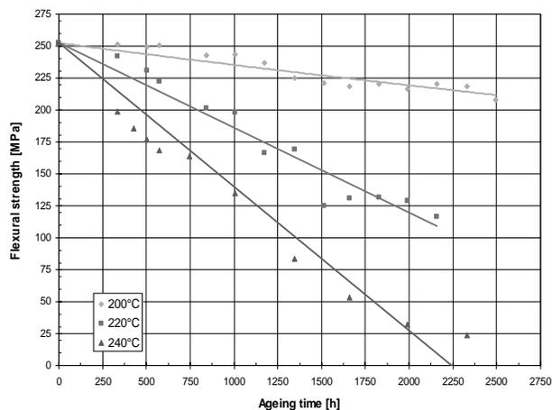
Fig. 13. Dependence of flexural strength on ageing time
