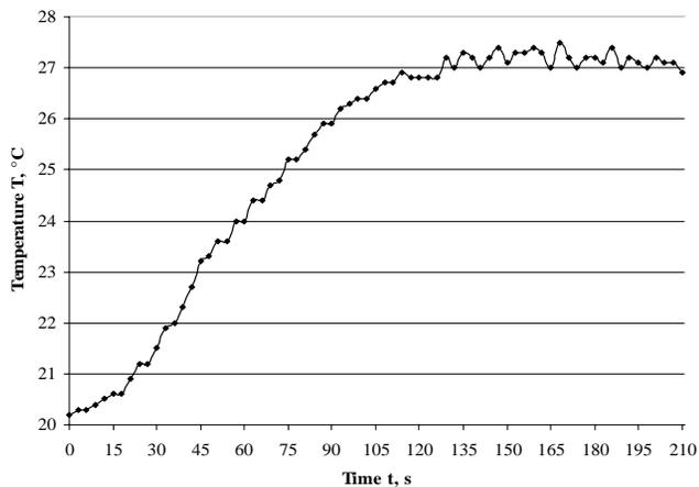
Fig. 6. Temperature – time dependence for central point of the sample aged 1992 hours in 240 °C
