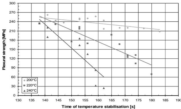
Fig. 9. Relation between flexural strength and time of temperature increase
