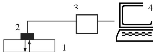
Fig. 11. Ultrasonic testing stand: 1) specimen, 2) ultrasonic head, 3) defectoscope, 4) computer system with software to results registering and analysis
