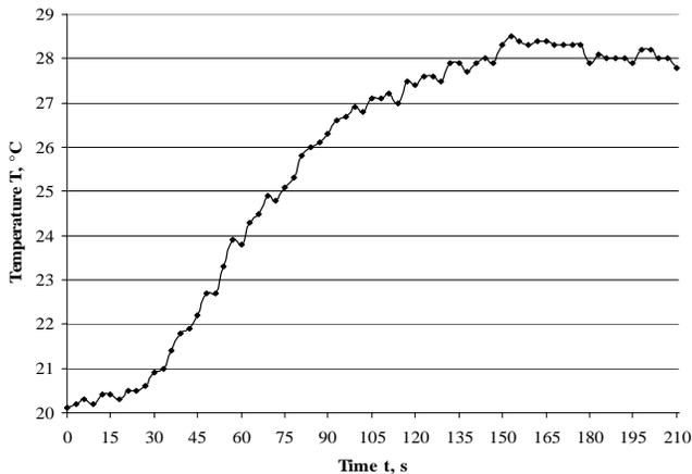
Fig. 5. Temperature – time dependence for central point of the sample aged 1992 hours in 200 °C
