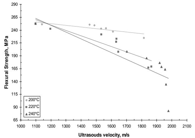
Fig. 14. Relationships between flexural strength and ultrasounds propagation velocity
