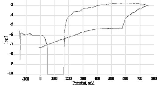
Fig. 8. Anodic polarization curve for grinded samples
