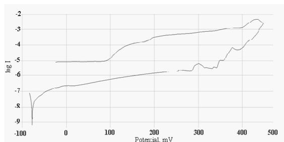
Fig. 12. Anodic polarization curve for grinded samples
