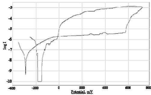
Fig. 4. Anodic polarization curve for grinded samples
