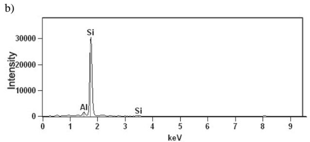
Fig. 5. a) The surface distribution of the alloying elements in the area of Si and “Chinese script” shaped inclusions occurrence; b) EDS X-ray spectra of the local analysis of rounded in shape particles
