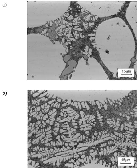
Fig. 9. The alloy microstructure after 20 min annealing at 580°C
