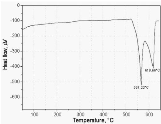
Fig.6. DSC curve of the AlSi5Cu2Mg alloy in the T6 conditions obtained by heating at the rate of 4°C/min to 625°C
