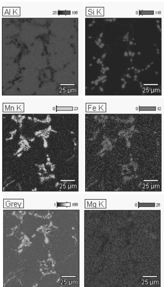
Fig. 4. The surface distribution of the alloying elements in the area of Si and “Chinese script” shaped inclusions occurrence
