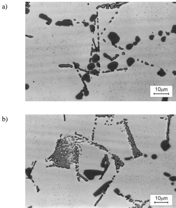
Fig. 7. The AlSi5Cu2Mg alloy microstructure after 20 minutes annealing at 518°C
