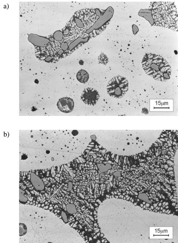
Fig.8. Optical micrograph of the AlSi5Cu2Mg alloy subjected to annealing at 568°C for 20 minutes
