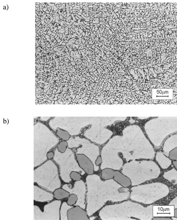
Fig. 10. The AlSi5Cu2Mg alloy microstructure after 20 minutes annealing at 629°C
