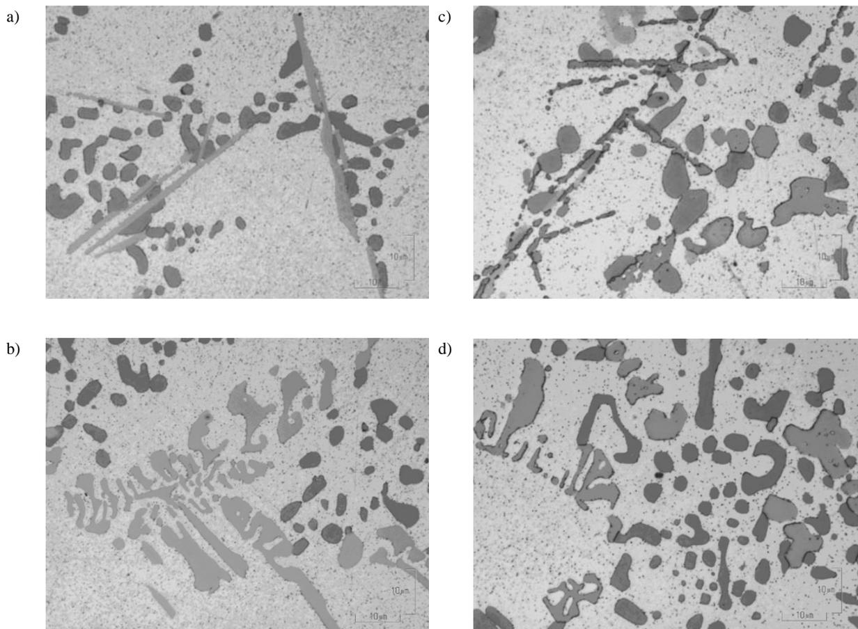
Fig. 2. Optical metallography pictures of the AlSi5Cu2Mg alloy in the T6 condition a, b) unetched; c, d) etched microstructure - images from light microscope (LM)
