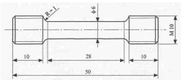
Fig. 2. Sample of tensile test at elevated temperatures
