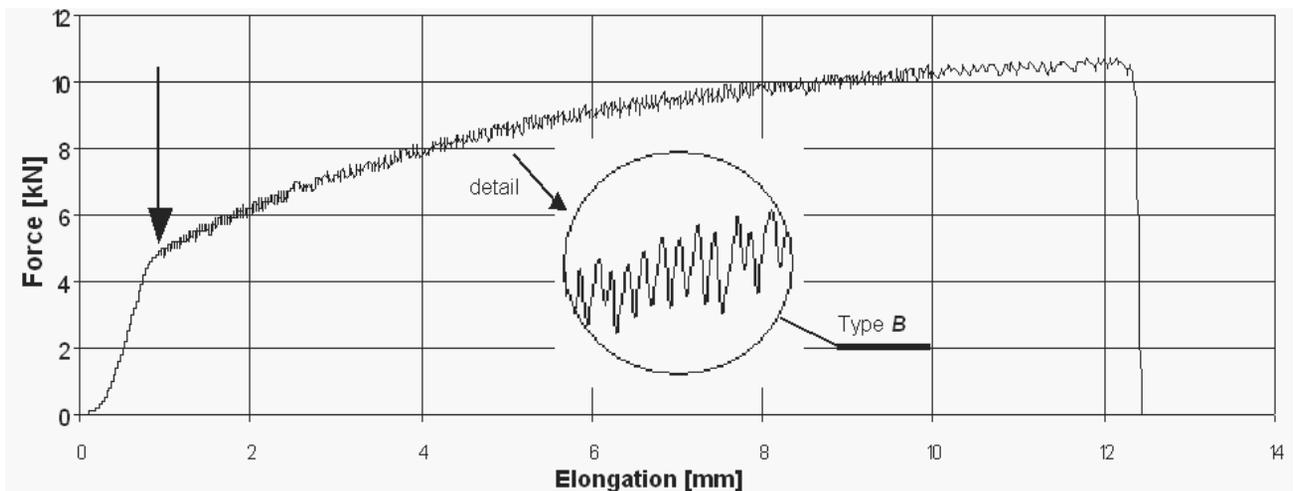
Fig. 14. Tensile stress-strain curve for CuZr0.05% alloy at 250°C
