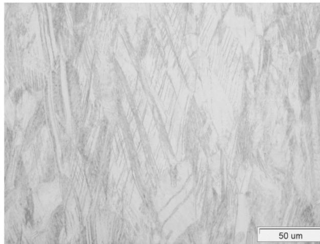
Fig. 7. Single – phase structure of bronze CuSn7 with the shear bands; tensile temp. 250°C, break–off zone of the sample; 500x
