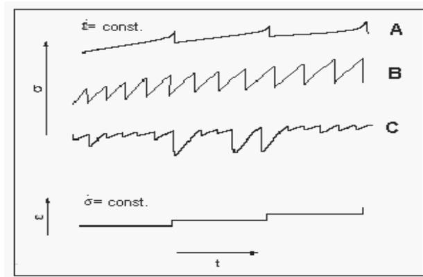
Fig. 1 Types of "teeth" characteristic for the heterogeneous deformation of the Portevin – Le Chatelier phenomenon [10]
