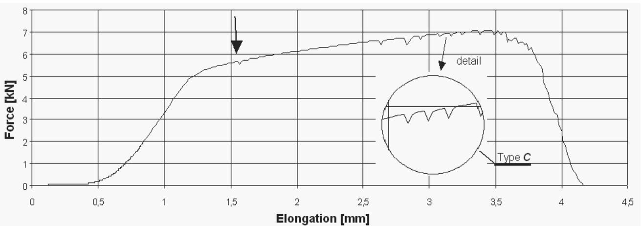
Fig. 11. Tensile stress-strain for CuSn7Zr0.05% alloy at 300°C
