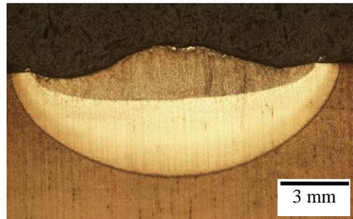
Fig. 4. Surface layer of the X40CrMoV5-1 steel alloyed with NbC powder, laser power 2.0 kW
