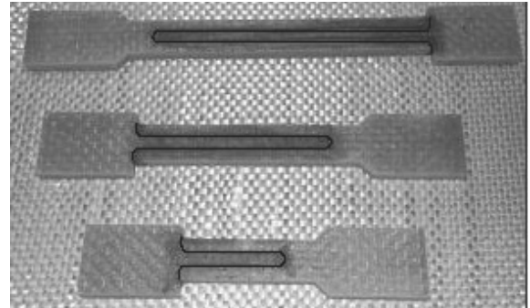
Fig. 2. Tongue and groove bonded joint configuration of 225 mm 150 mm and 75 mm
